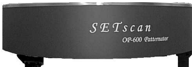
Figure 5. Photograph of the SETScan optical patternator.
