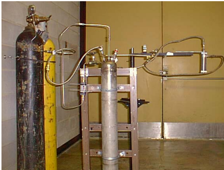
Figure 4. Photograph of the high pressure spray system.
