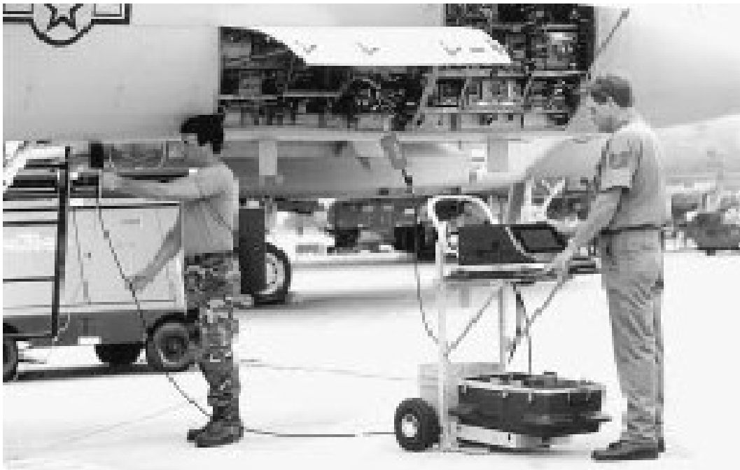
Figure 30 – Technicians (Non RSAF) Loading Data File to the Aircraft Using EDNA
