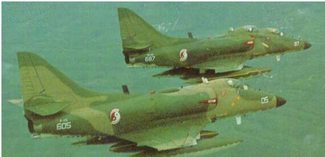
Figure 24 - A Pair of Skyhawks In Formation. Aircraft 687 is a TA-4S Advanced Trainer With a Separate Canopy for the Instructor, a Feature that Makes the RSAF's TA-4 Unique in the World [From 12]
