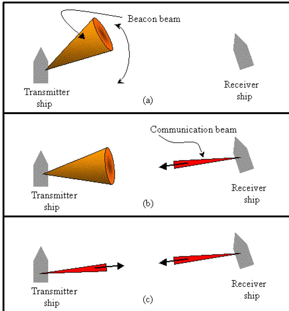
Figure 29. Using beacon beam for acquisition and pointing
