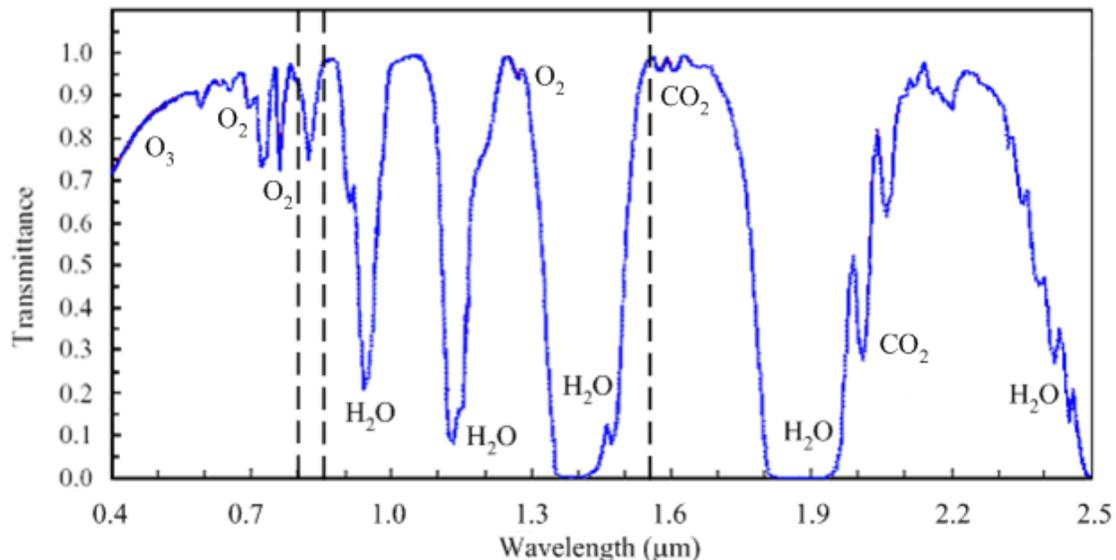
Figure 11. Visible and Infrared Atmospheric Transmittance (From: [Neo 2003])
