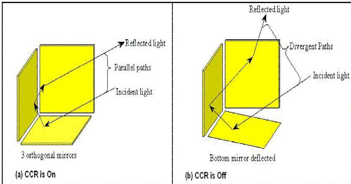
Figure 31. Modulated Corner Cube Reflectors (After: [Sporian 2004])
