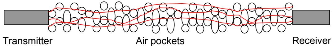
Figure 16. Effect of scintillation on a laser beam
