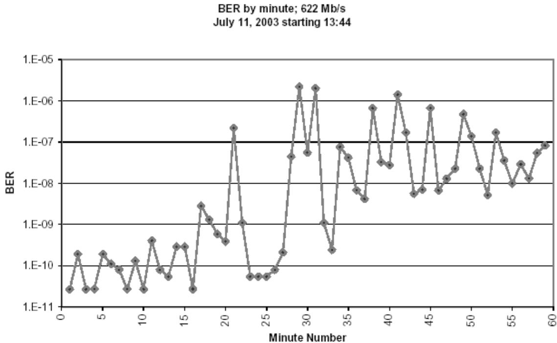
Figure 10. BER test 2. (From: [Vilcheck 2003])
