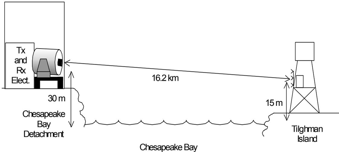
Figure 4. Chesapeake Bay Testbed Geometry (From: [Vilcheck 2003])
