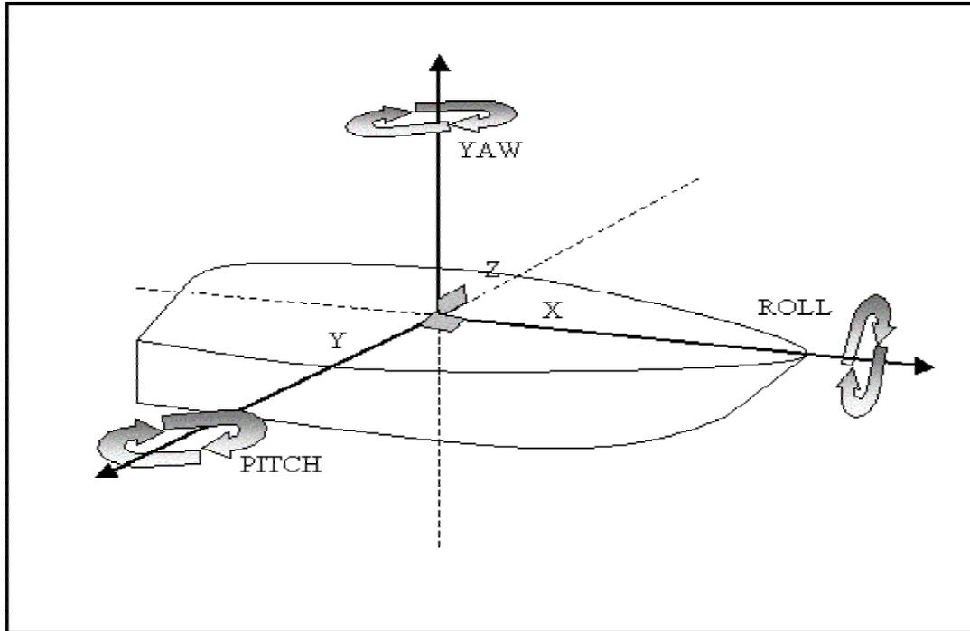
Figure 26. Ship motions: yaw, pitch, and roll
