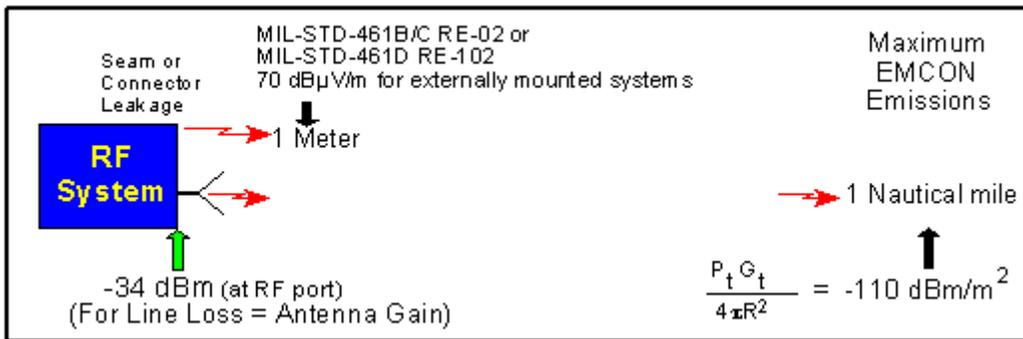
Figure 25. EMCON Field Intensity/Power Density measurements (From: [NAWCWD 2004])
