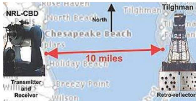
Figure 6. NRL-CBD to Tilghman Island FSO lasercomm test bed. Bistatic transmitter and receiver at CBD (left) and corner-cube retro-reflector arrays mounted on the tower on Tilghman Island (right) (From: [NRL 2004])
