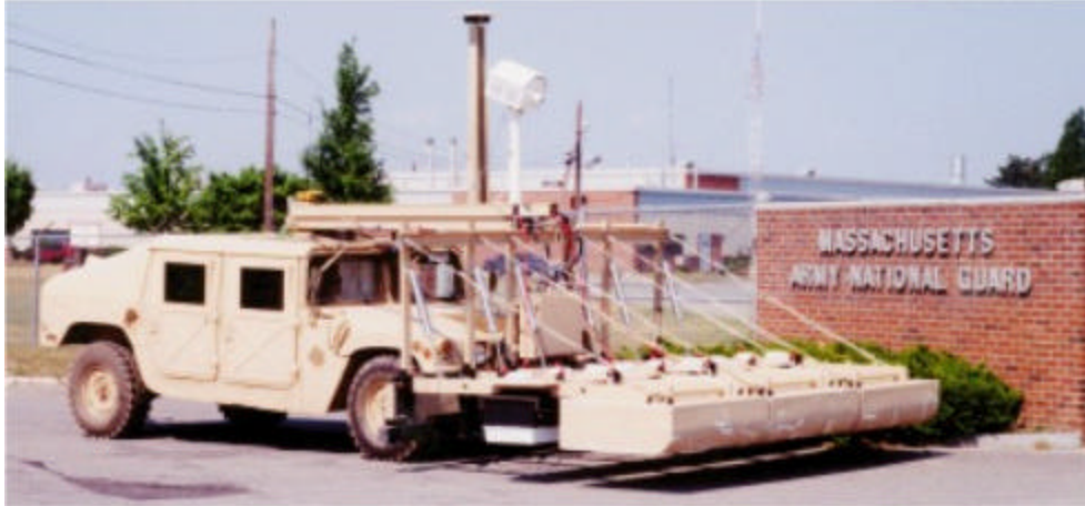
Figure 8. GPR in service with the U.S. Army Corps of Engineers (from [20]).
