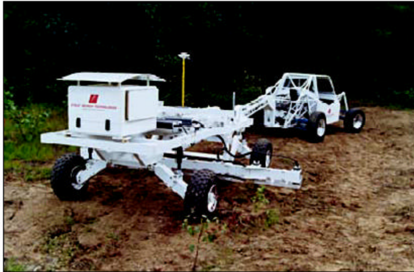
Figure 2. A digital geophysical mapping system for detection of UXO (from [2]).
