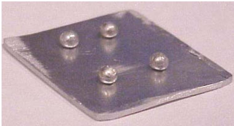
Figure 10. Composite solder balls of ~1mm diameter on an aluminum substrate following surface cleaning.
