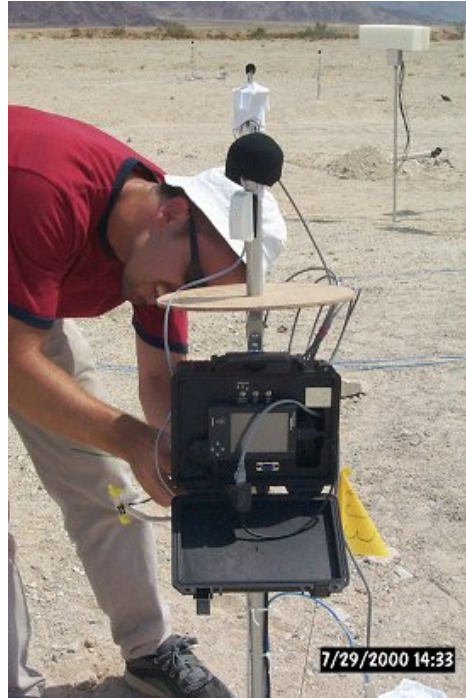
Figure 14. WINS NG 1.0 node as setup and left for 2 weeks during SITEX00.
