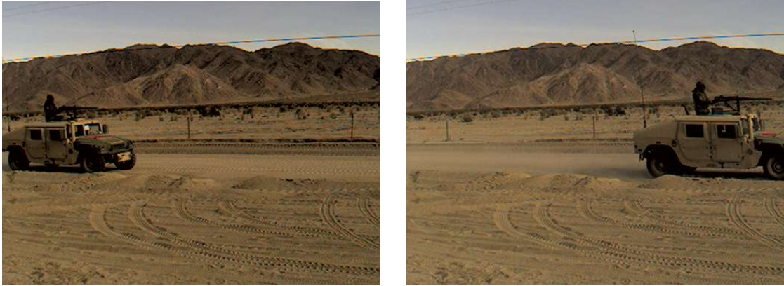
Figure 41. Imager 1 captures HMMWV with automatic weapon in time sequence image pair. Note that image sequence offers two viewing angles and backgrounds, rendering the weapon more visible in the second image. (From 6 Dec 2001 image database.)
