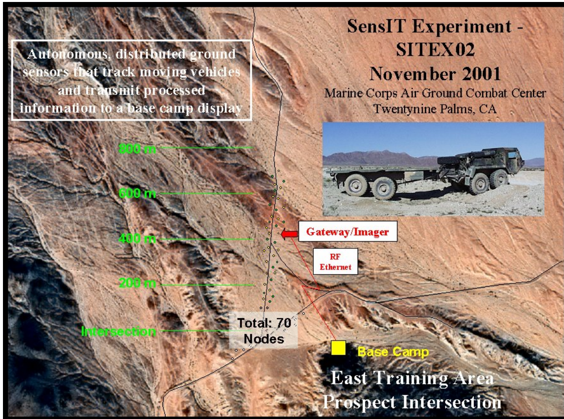
Figure 52. Node layout, aerial map, and overview of the SITEX02 Experiment using 70+ WINS NG 2.0 nodes.
