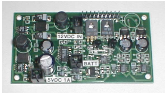
Figure 5. The WINS NG Power Supply. The WINS NG Power Supply is a low power system intended to support a multiplicity of sensors and interfaces with both low average power, and high peak power performance.
