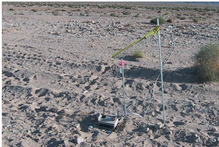
Figure 51. WINS NG 2.0 node deployed at SITEX02. The large pole with caution tape was used to mark the location of the node to prevent it being run over.
