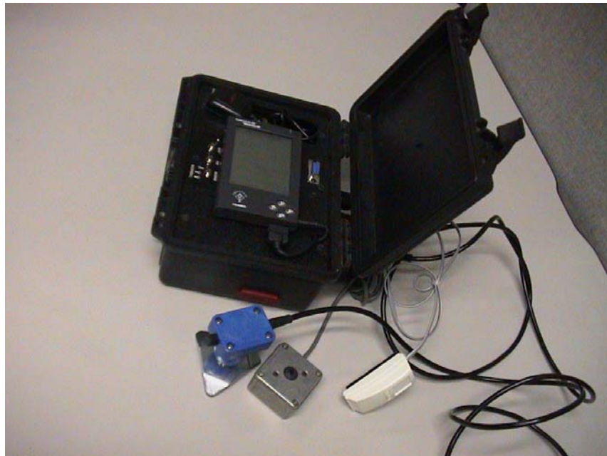
Figure 10. The WINS NG environmentally resistant package. Sensors are placed external to this package for optimal performance.
