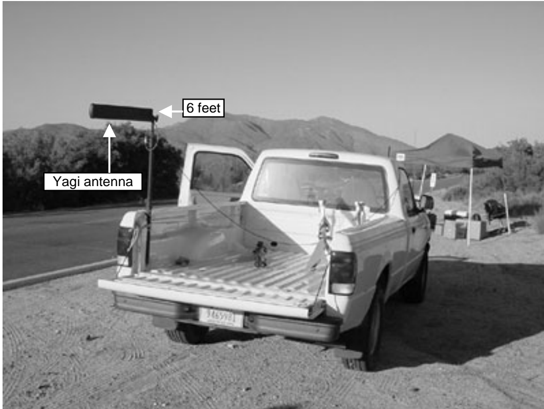
Figure 10. Mobile Receiver Station in Field Range Test (Simulated OCU)
