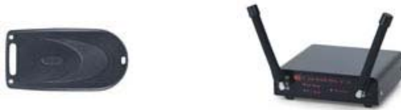
Figure 4. Spider III RFID tag and tag reader for Product Assessment System payload
