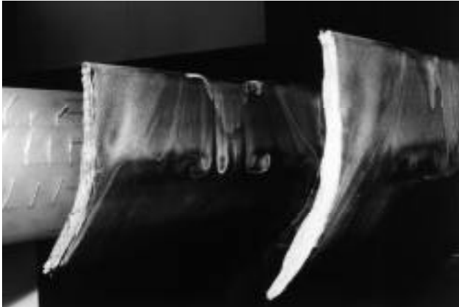
Fig. 7 Surface flow visualization at 380,000 Reynolds number and 38° inlet flow angle.
