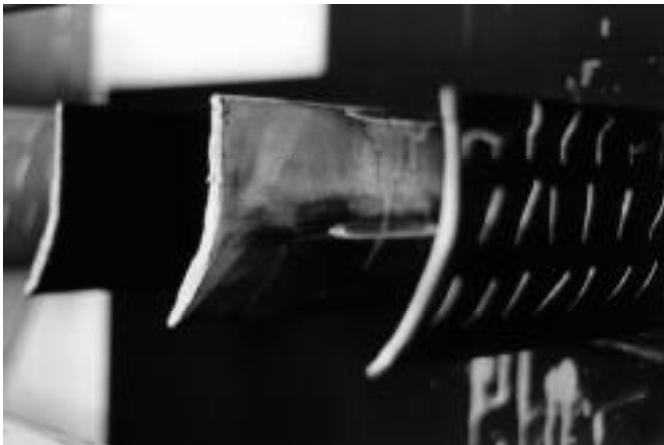
Fig. 8 Surface flow visualization at 210,000 Reynolds number and 38° inlet flow angle.
