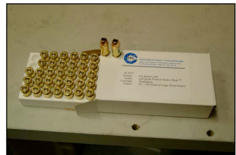
.45 ACP Ammunition Using Recovered Processed Navy Gun Propellant
