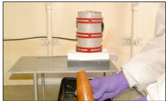
TNT Slug from Induction Heating
