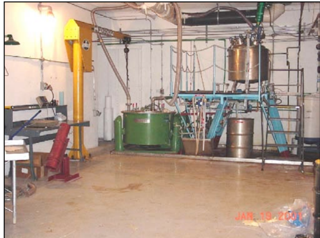
Sub-scale HMX Recovery Plant
