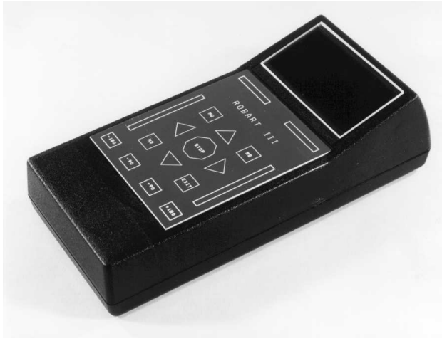
Figure 3. A capacitive touch-panel interface on the hand-held pendent mimics the drive icons shown in Figure 2.
