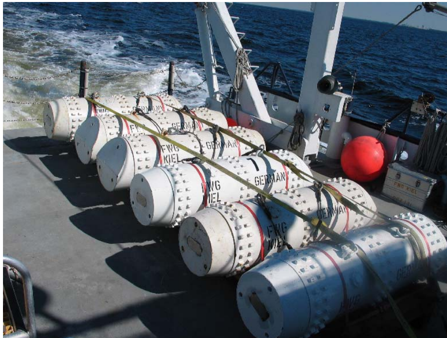
Figure 6. Six FWG Instrumented Mines.
