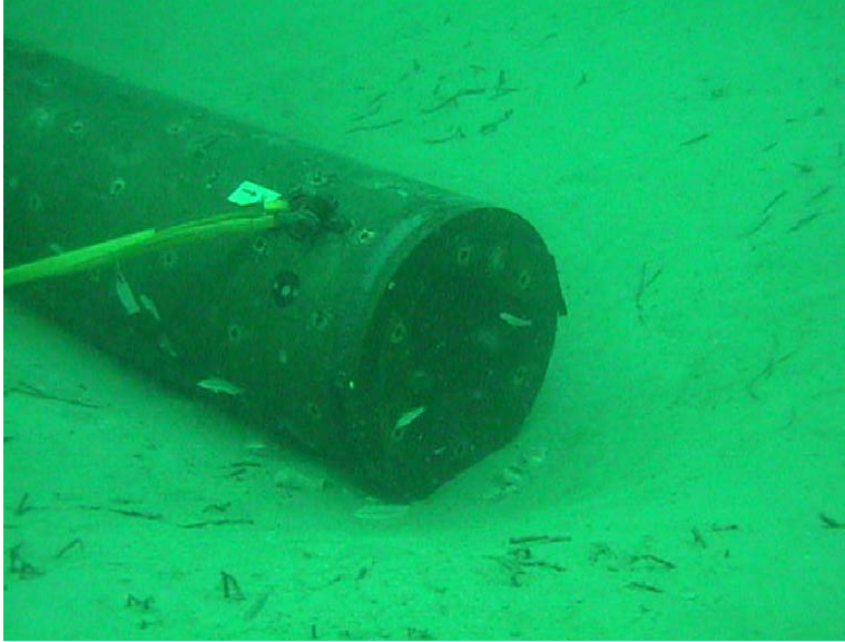
Rear view of AIM # 3 at recovery— note worm tubes and scour pit
