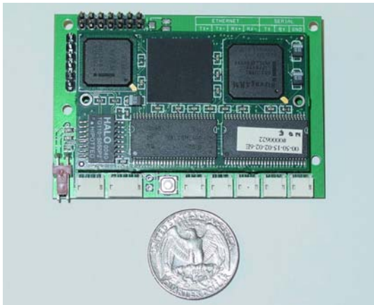
Figure 3. A nanoEngine and its daughterboard.
