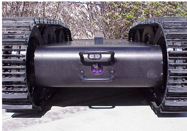
Figure 5. Rear of the robot showing the carrying/recovery handles, rear-facing camera, and ON/OFF switch.
