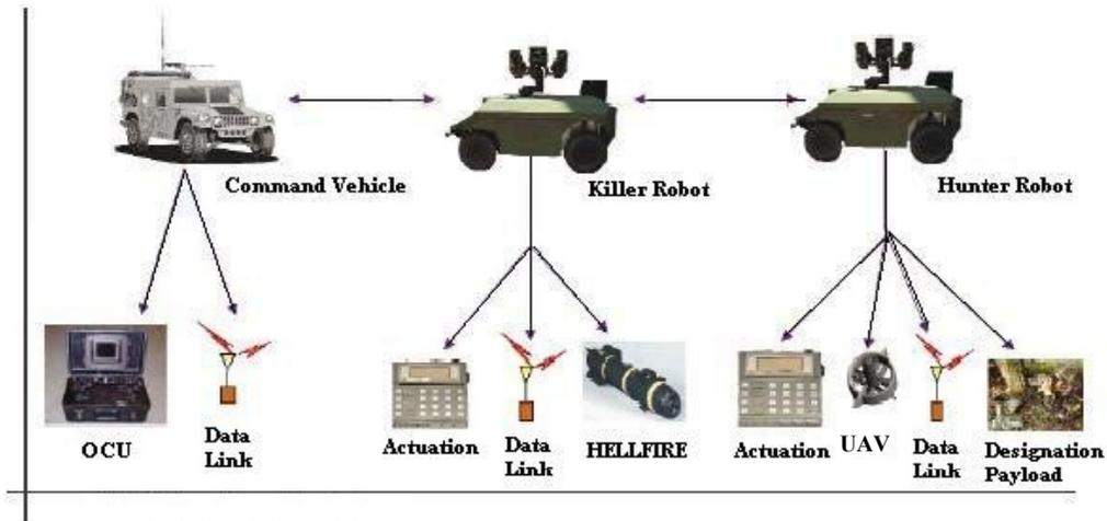
**Figure 2. COUGAR Phase II Demonstration System**
