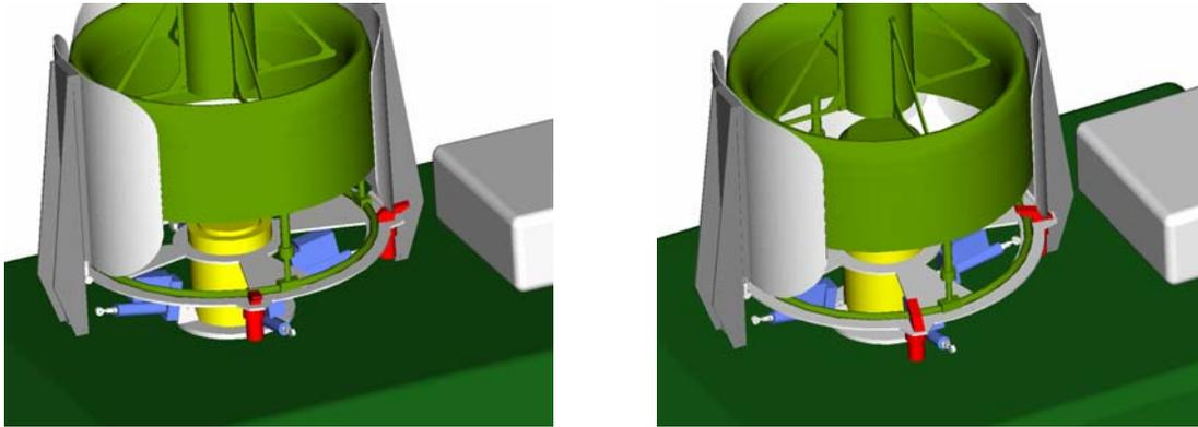
**Figure 8. Rotating Finger Latches**
