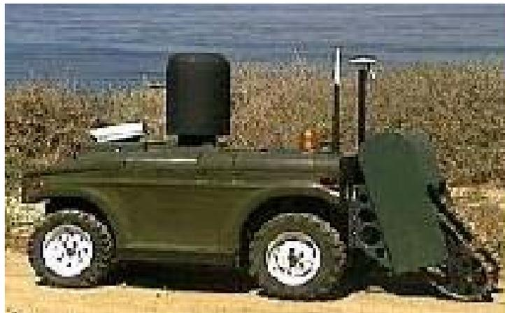
**Figure 1. MDARS-E with Marsupial Delivery System**
