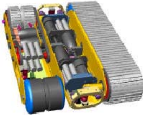
Figure 3. Cutaway of the Novel UGV showing components.
