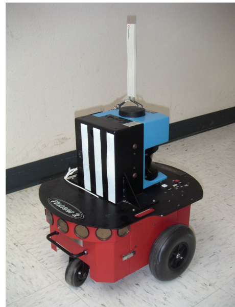
Fig. 4. A relay node with retroreflective barcode beacon. This barcode is the number 21 (10101 in binary).
