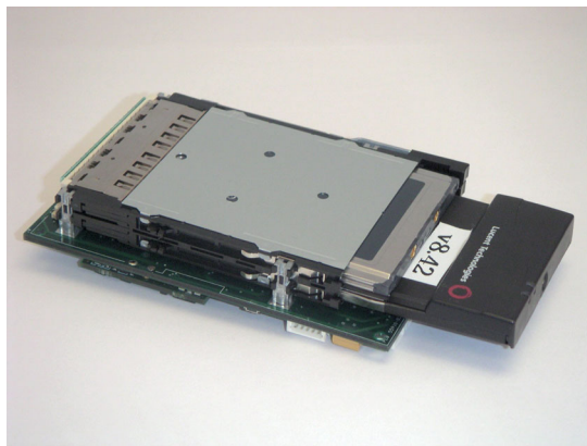
Fig. 3b. The other side of the RIB2, showing two PC Cards
