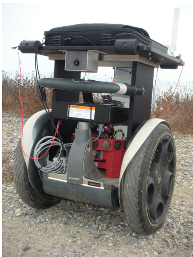
Fig. 2. The Segway RMP configured as a lead robot.
