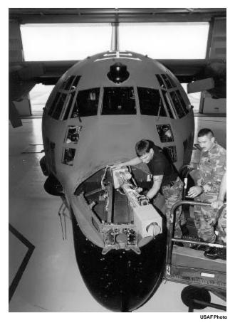
The Skyanchor is removed from the nose section as the STARS is officially retired from the Air Force.
