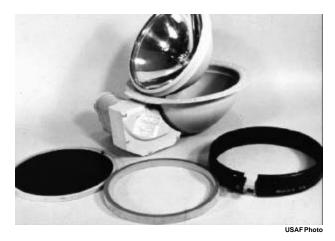
IR landing light modification. The double retaining ring is on the right, and the IR lens is on the left.
