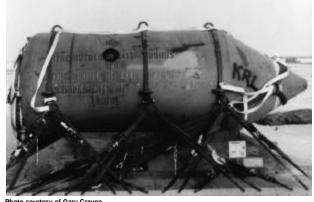
A BLU-82B rigged for airdrop. The extended nose fuse
