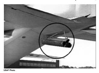
Two ASROC rockets were mounted near the aft beavertail and prevented over rotation during takeoff.
