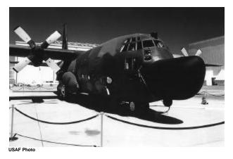
The new Combat Talon II has an extended radome and chin-mounted FLIR turret. The large radome is required to accommodate both the FLIR and the AN/APQ-170 radar.
