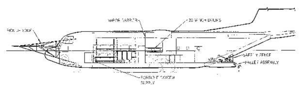
Figure 3. C-130A/B Fulton Skyhook Installation (Internal View) (Source: Lockheed Aircraft Corporation, ER-4112, 8 February 1960.)
