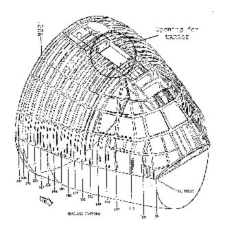
Figure 22. Forward Fuselage—Upper Structure with UARRSI Opening (Source: Illustration provided by Detachment 4, 645th MAS, Palmdale, Calif.)
