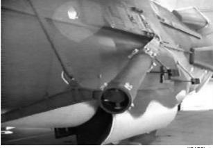
Eight Mark 56 rocket motors (four on each side) were mounted on the aft rear fuselage area and were pointed rearward at a 45-degree angle.
