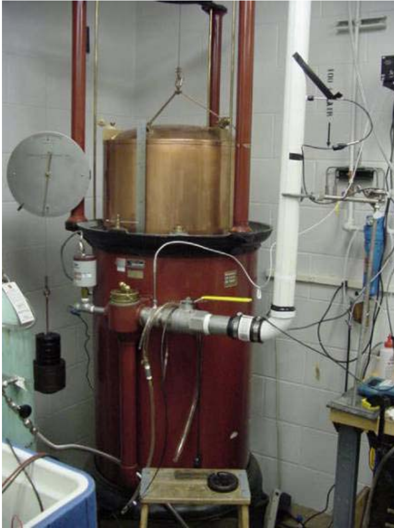
Figure C-5. Bell Prover with TSI Air Velocity Transducer
