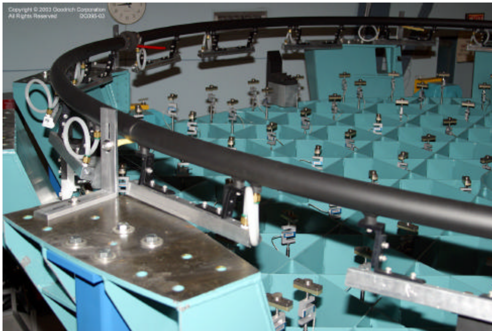
Figure 8. Primary mirror cell showing the actuators ready for bonding and the laminar airflow system (dark ring).
