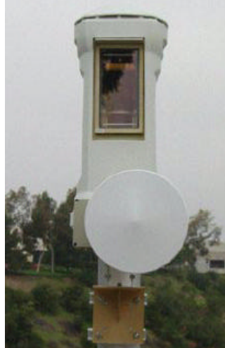
Figure 33. Airfiber's Hybrid FSO/Radio with a 13-inch Parabolic Dish for Microwave Transmission (From: [Bloom 2003])
