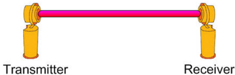
Figure 12. An ideal transmission with no divergence
