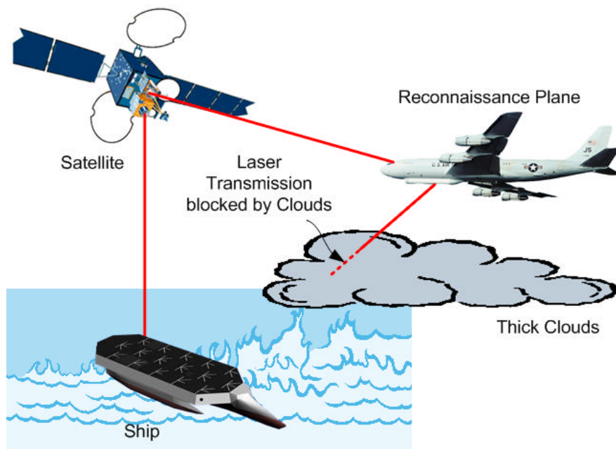
Figure 35. Effective Spatially Diverse FSO Links
