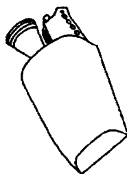
ORBITAL MANEUVERING SYSTEM (OMS)/REACTION CONTROL SUBSYSTEM (RCS) MODULE (TYPICAL) - Skin and Stringer - Graphite Epoxy and Milled Skin - Titanium Thermal Barrier
