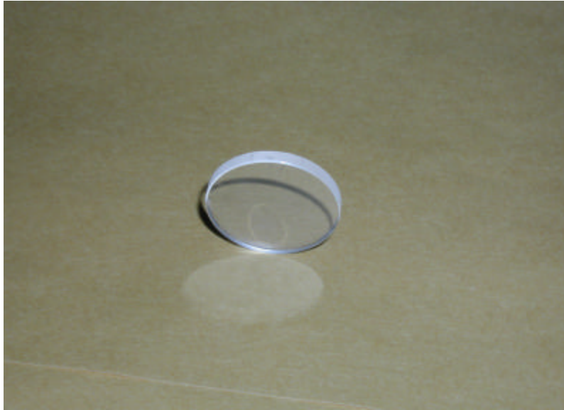
Figure 5. A photograph of the testing material, single crystal of aluminum oxide.
