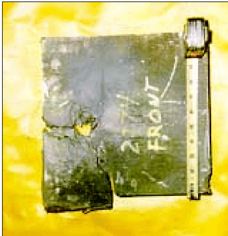
Figure 2. Severe spall of unconfined back surface due to ballistic impact on finite thickness titanium armor plate.
