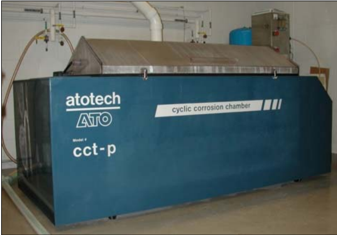
Figure 2. Test chamber configuration used for GM 9540P.
