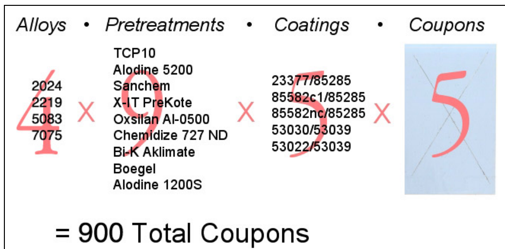
Figure 1. GM 9540P test panel matrix breakdown.
