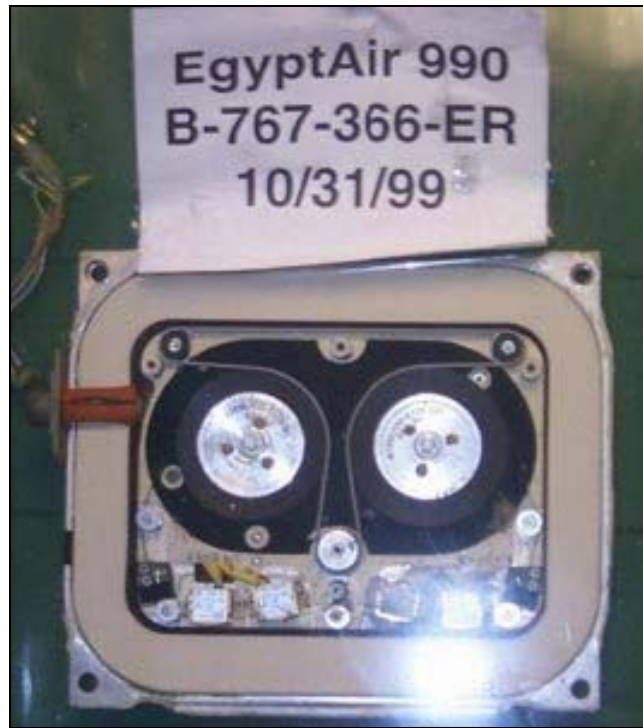
Figure 6. EgyptAir 990 Cockpit Voice Recorder
