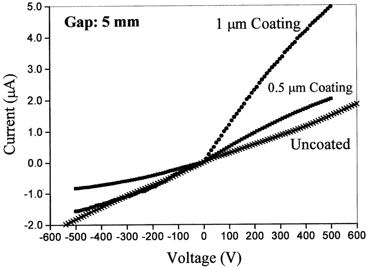
**Figure 13.** Current-voltage characteristics measured in the dark for an uncoated sample and two samples of diamond-coated GaAs switch substrate with a gap setting of 5 mm.
