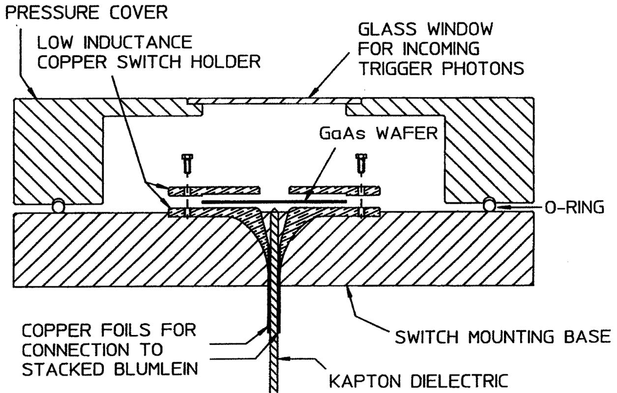
**Figure 17.** Schematic drawing of the cross section of the switch assembly used in this work for switch longevity tests.
