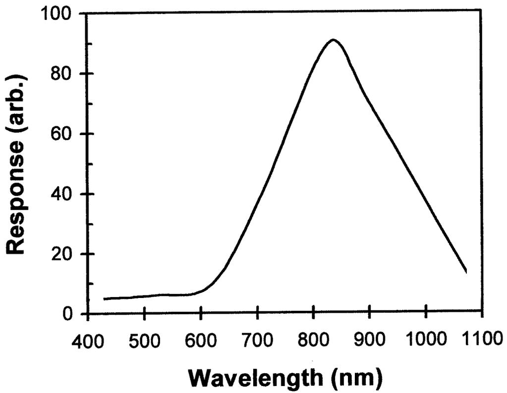
**Figure 8.** Spectral response for an amorphous diamond/ Si heterojunction operated under the reverse bias at 50 V.
