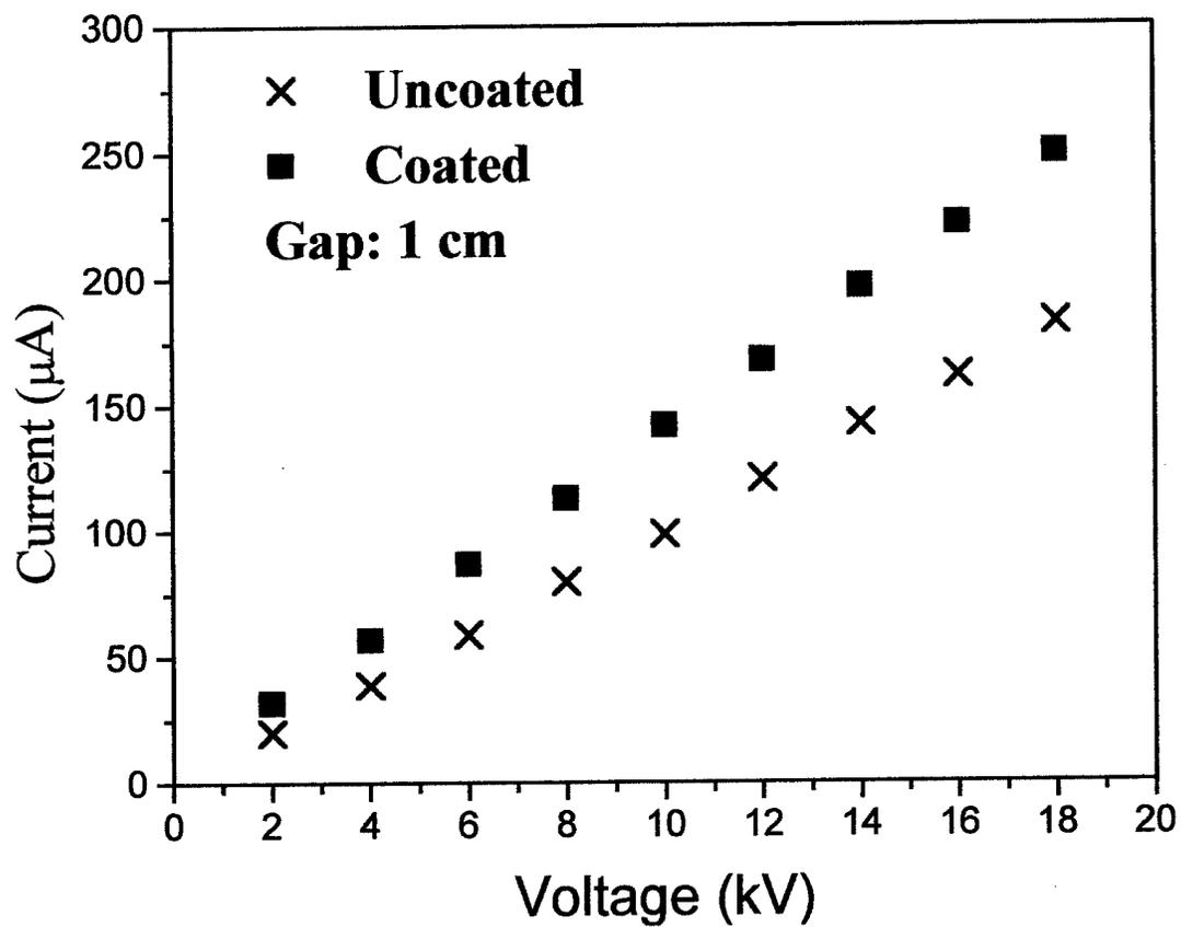
**Figure 15.** High voltage I-V characteristics measured in the dark for an uncoated sample and a sample of diamond-coated GaAs switch substrate with a gap setting of 10 mm.
