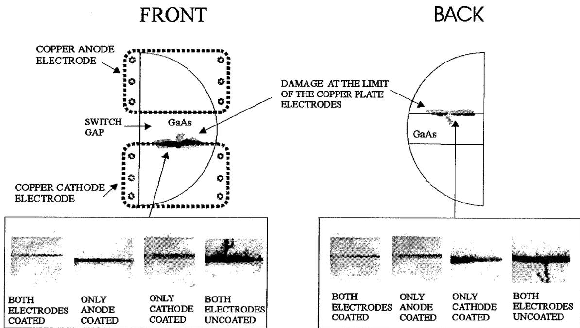
**Figure 18.** Schematic drawing of the appearance of damage on both sides of switch used in these studies. For comparison the negative photographs of the switch electrode areas for diamond-coated and uncoated switches are shown after  $1 \times 10^4$  commutation cycles.
