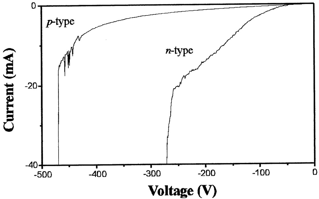
**Figure 9.** Current-Voltage characteristics showing the breakdown voltages for the nominal amorphous diamond films on p- and n-type Si substrates. Measurements performed in the dark under reverse bias conditions.
