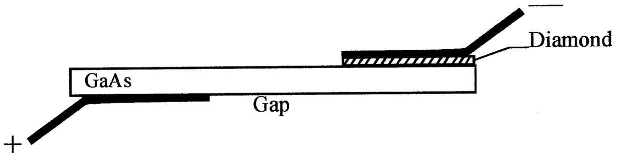
**Figure 11.** Schematic presentation of a switch sample cross section used for forward I-V measurements.
