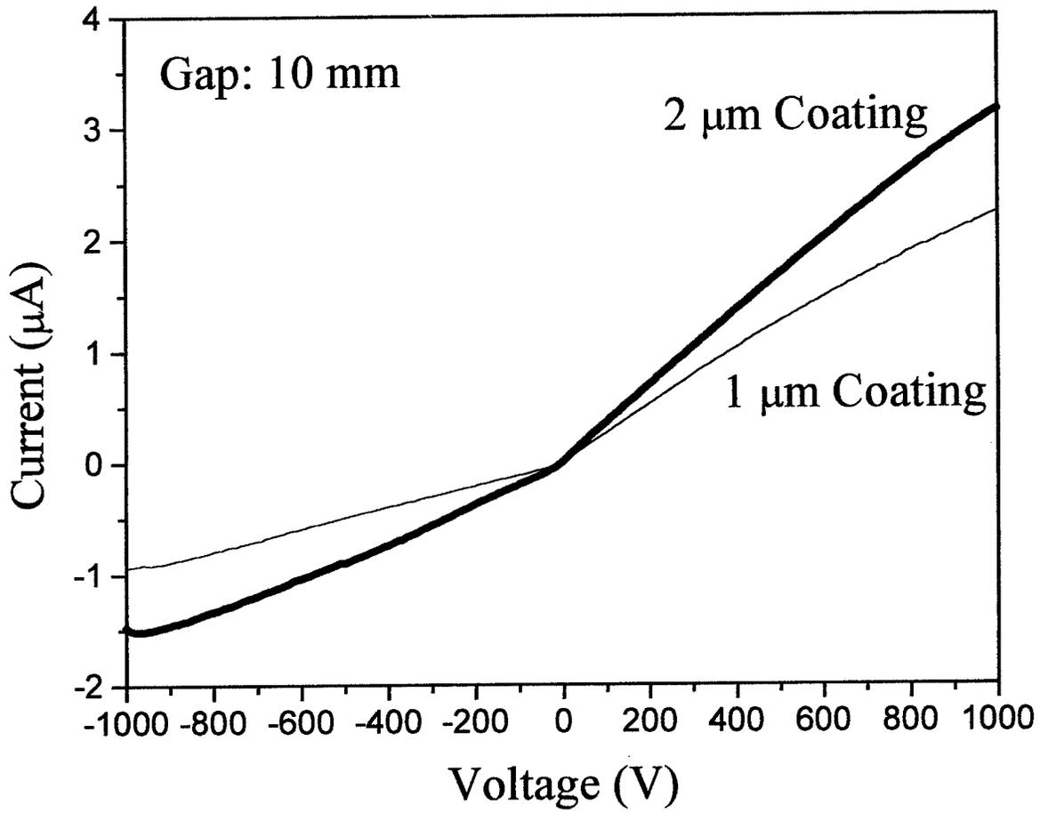
**Figure 14.** Current-voltage characteristics measured in the dark for two samples of diamond-coated GaAs switch substrates.
