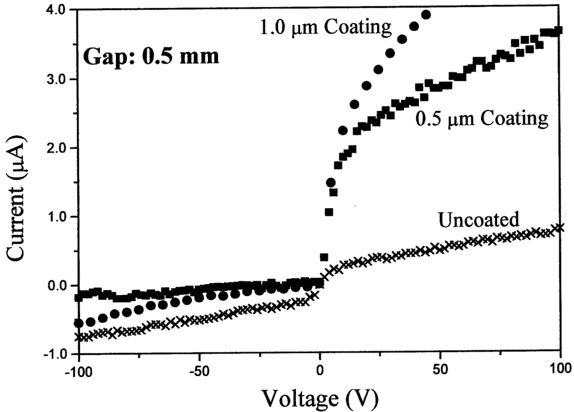
**Figure 12.** Current-voltage characteristics measured in the dark for an uncoated sample and two samples of a diamond-coated GaAs switch substrate with a gap setting of 0.5 mm.
