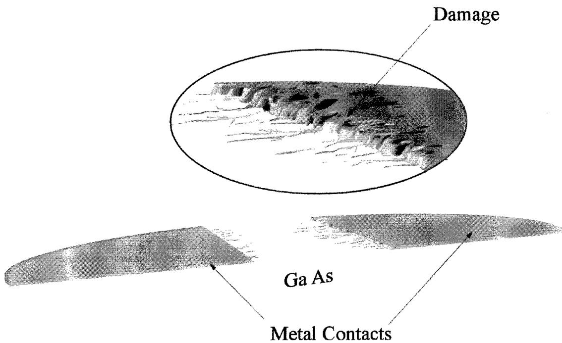
**Figure 5.** Schematic presentation of a GaAs high gain photoconductive switch with conventional metal contacts. Damage due to high current filaments is shown in the switch gap and metal electrode contact areas.
