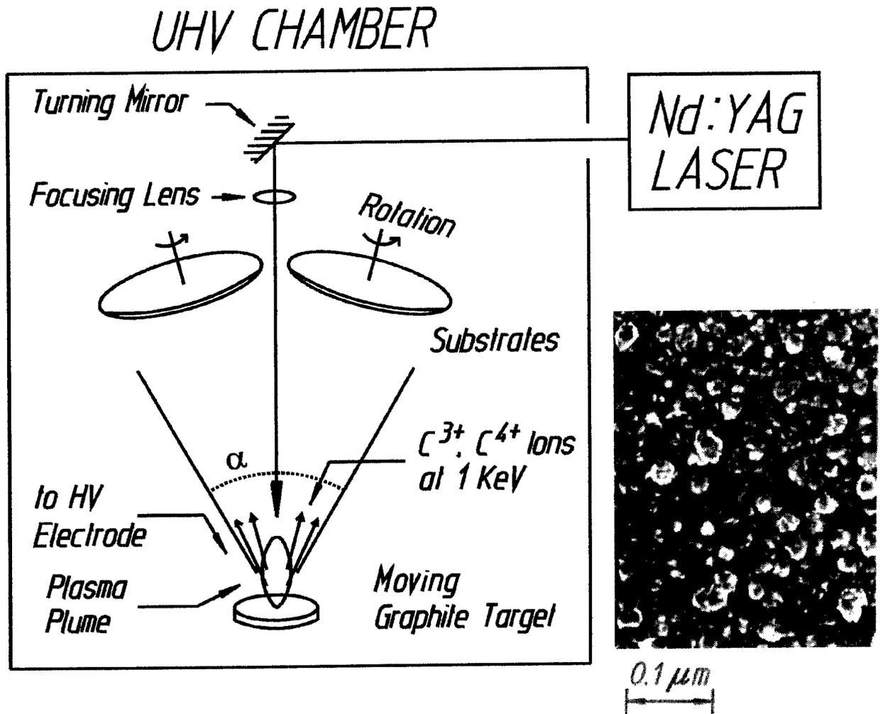
Figure 6. Schematic representation of the laser plasma discharge source used in this work to prepare amorphous diamond coatings. Diamond nodules are also seen in an image produced by TEM of a gold-coated replica of a film of amorphous diamond.
