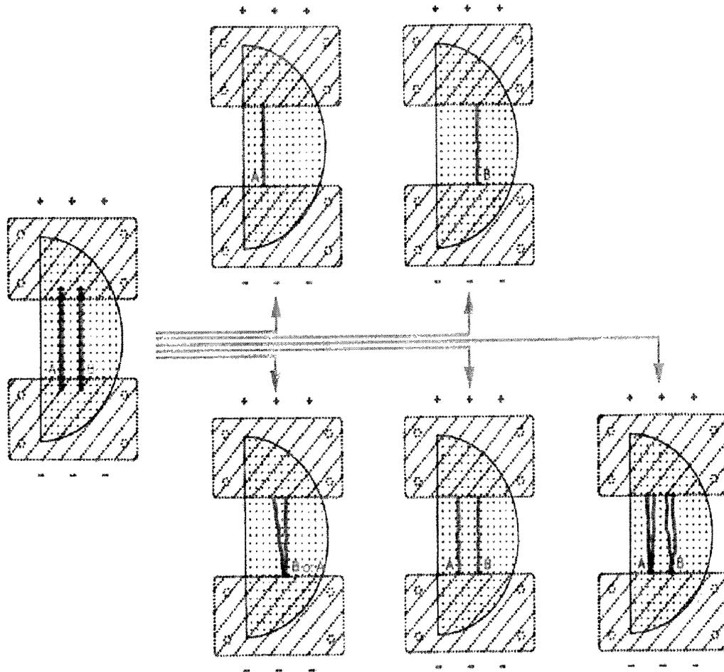
**Figure 4.** Schematic diagrams of a laser diode beam focused on the switch in two lines, and current filamentation seen with an infrared viewer.
