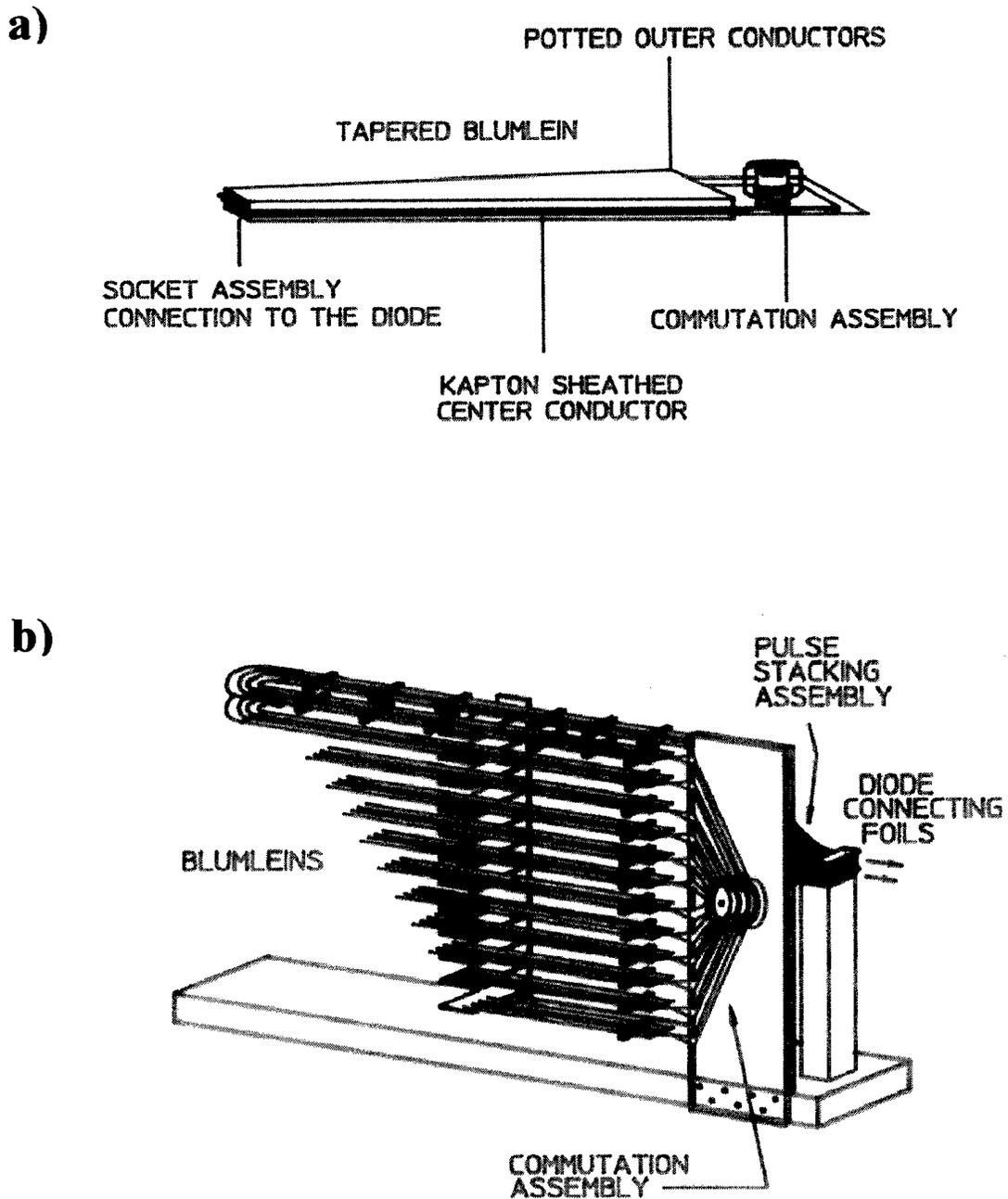
**Figure 1.** Schematic drawings of the high repetition rate, Blumlein pulse power generators developed at University of Texas at Dallas. (a) Pulse generator with a single traxial Blumlein pulse forming line. (b) Pulse generator with several Blumlein modules connected in parallel at switching end and stacked in series across the load diode.
