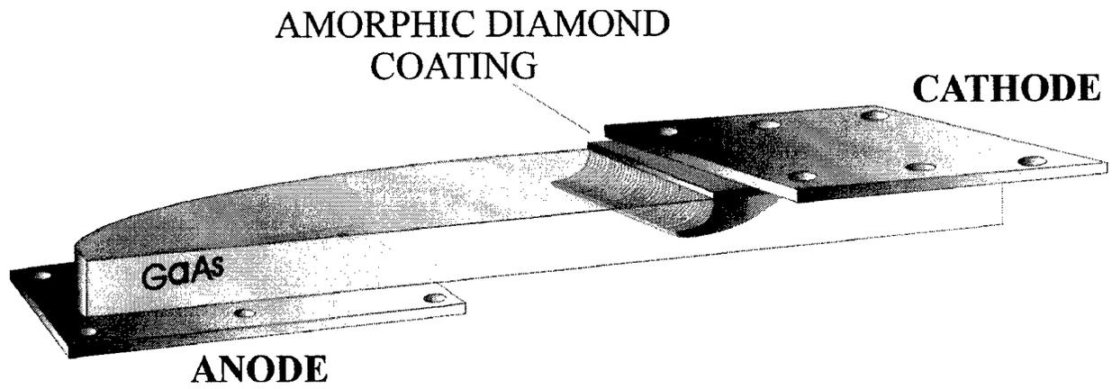
**Figure 19.** Schematic presentation of the switch/electrode assembly in an opposed configuration showing the off-state carrier movement due to the tunneling of electrons from amorphous diamond to GaAs.
