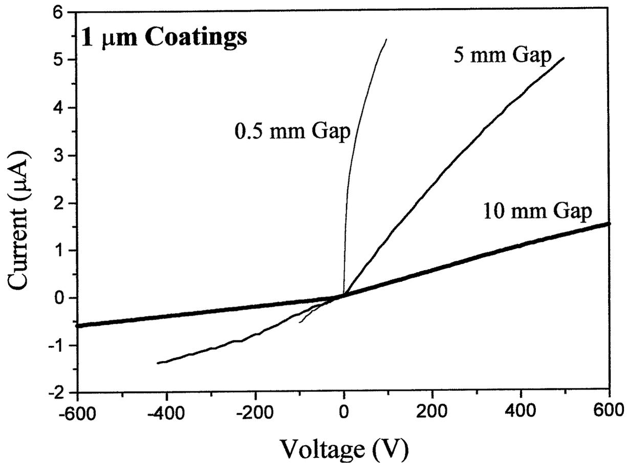
**Figure 16.** Current-voltage characteristics measured in the dark for three samples of diamond coated GaAs switch substrates with gap settings of 0.5, 5 and 10 mm.
