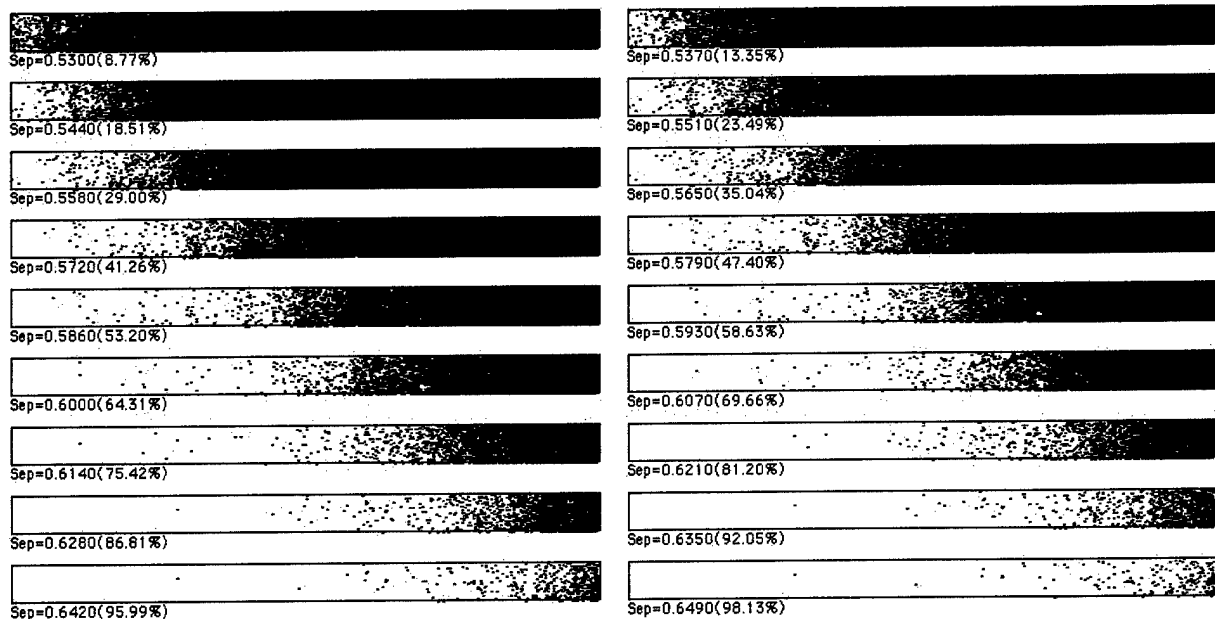
Figure AI-15. Fractured area projection plots (FAPPs) indicating the progression of the crack front.
