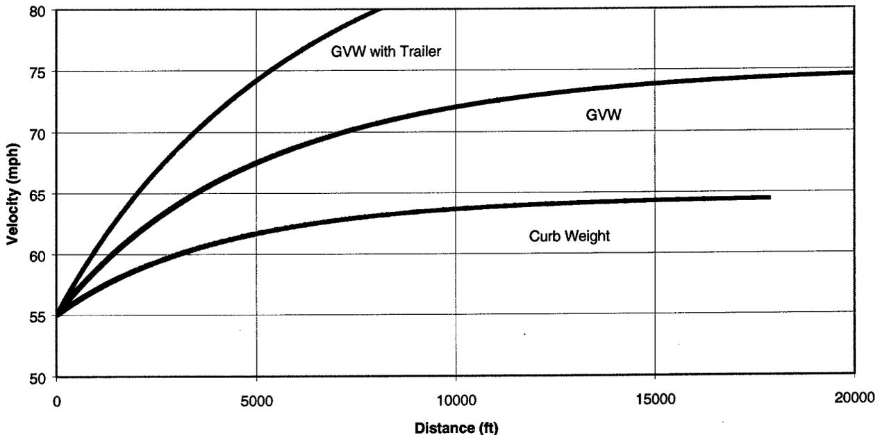
It can be seen that an LMTV at GVW, can easily achieve 70 mph on grades found on the US interstate highway system. The AØ vehicles were built with no engine braking hardware. The A1 vehicles have an engine exhaust brake, which can be turned off by the driver. This analysis is representative of all AØ vehicles as well as the A1 vehicles with the exhaust brake off. The use of a trailer further increases speeds.
