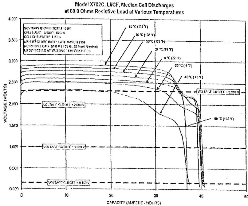
Figure 4: Capacity vs temperature of a Li/CF battery.
