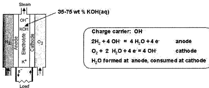
Figure 9: Alkaline H<sub>2</sub> Fuel Cell
