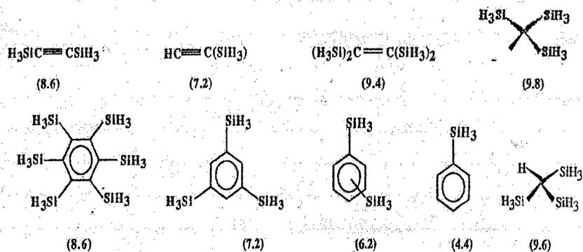
Figure 22: Proposed silanes and theoretical  $H_2$  mass fractions (in parenthesis).
