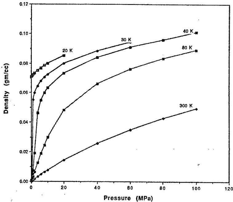
Figure 19: Density vs Pressure of Gaseous H<sub>2</sub>.
