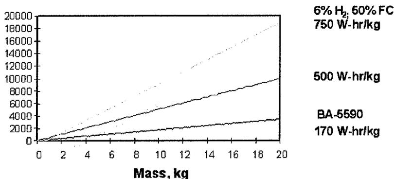
Figure 20: Energy vs mass of stored H<sub>2</sub> with a PEM Fuel Cell vs batteries and hybrid battery packs.
