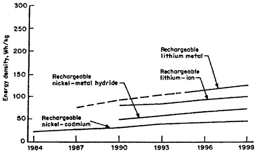
Figure 1: Battery performance characteristics.
