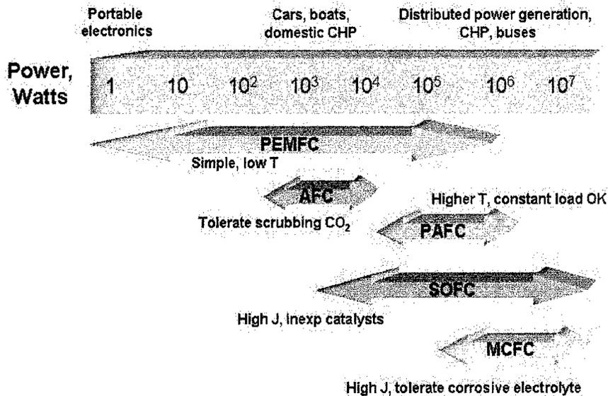
Figure 17: Range of fuel cell applications.
