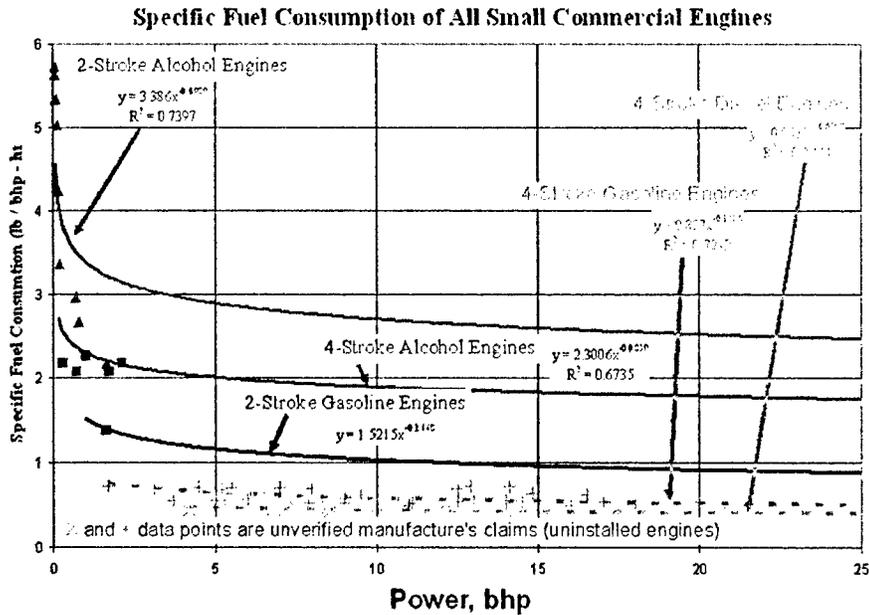
Figure 34: Specific fuel consumption of small engines
