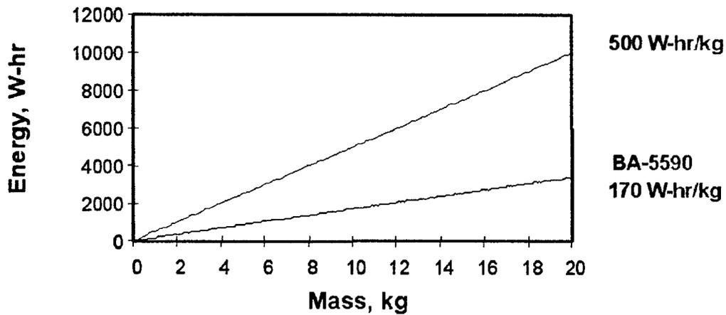
Figure 5: Energy vs mass of Li/CF and Li/SO<sub>2</sub> batteries.
