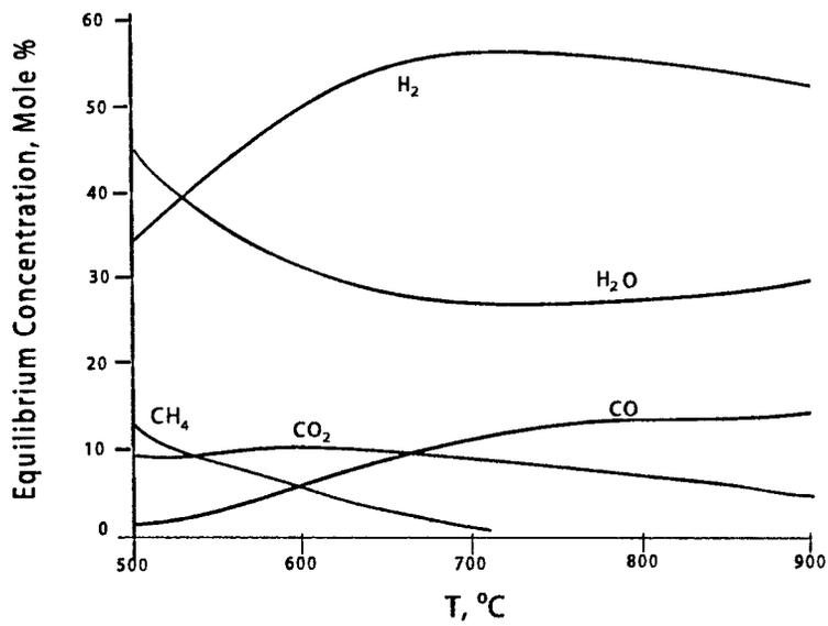
Figure 25: Composition of CH<sub>4</sub> steam reformat vs temperature.
