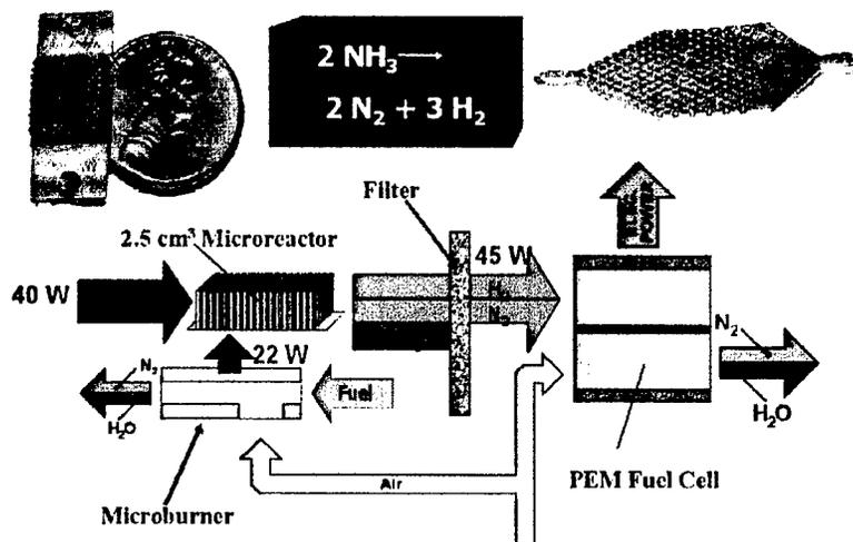
Figure 28: NH<sub>3</sub> cracking for hydrogen production.
