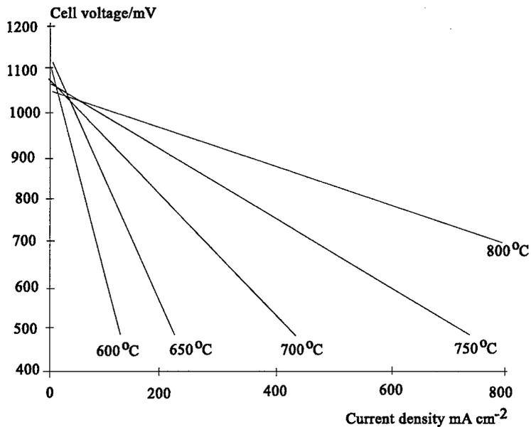
Figure 16: Solid oxide fuel cell performance versus temperature.
