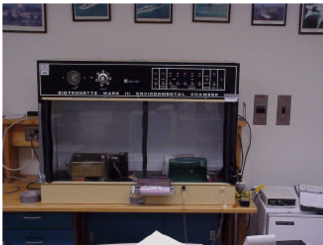
Figure 5.1: Environmental chamber with 3500 model reader.
