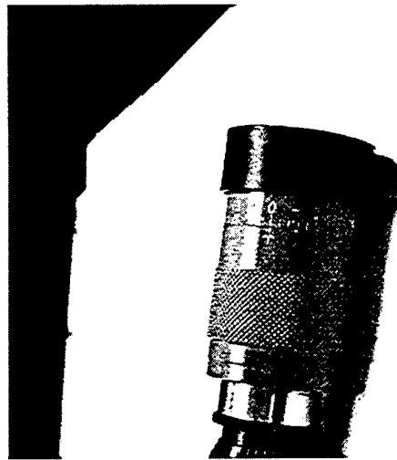
Figure 2. Dioptrimeter used to measure eyepiece settings
