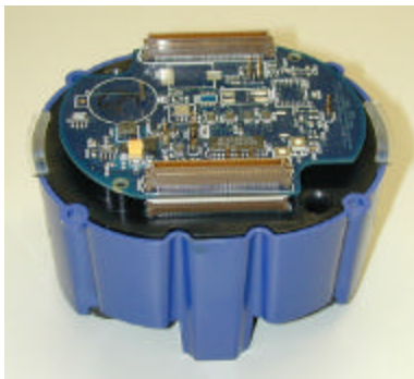
Node with final case. Sensor board is on top.
