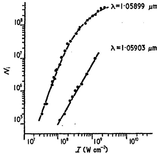
Data for photoionization of Cs for two laser wavelengths
