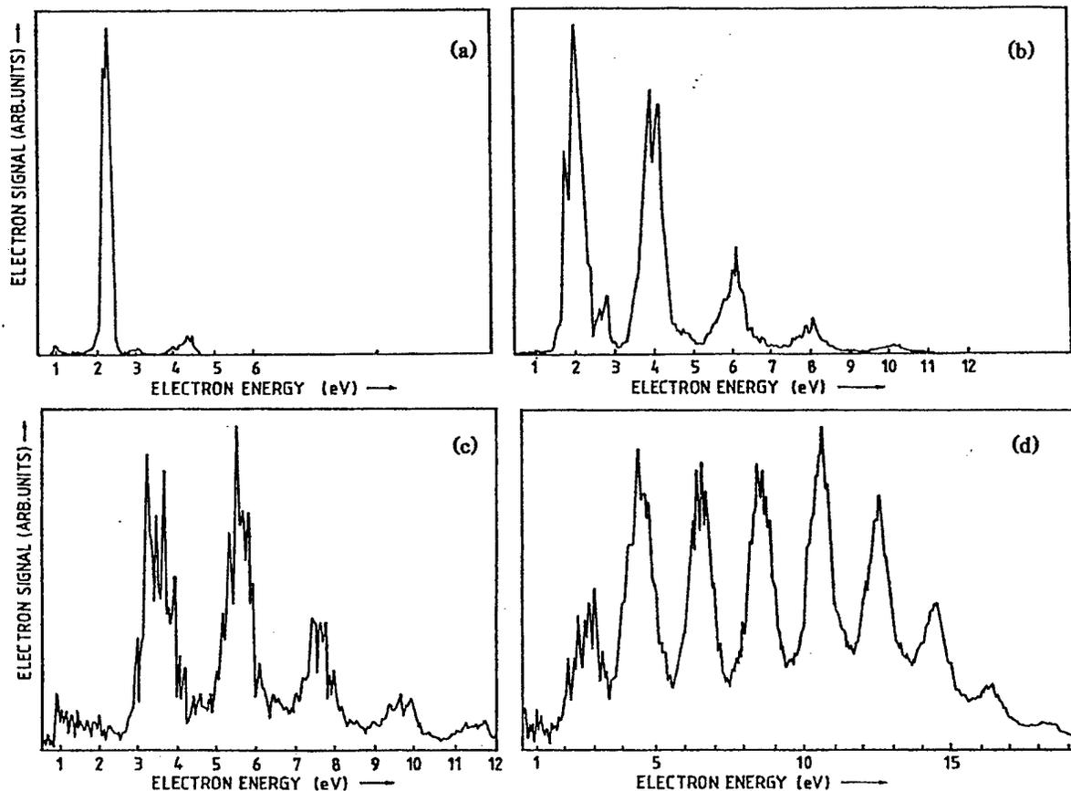
Electron energy spectrum measured after multiphoton ionization of xenon with 2 eV photon pulses of 100 fs duration. The pulse energies are a)  $11\mu\text{J}$ , b)  $24\mu\text{J}$ , c)  $29\mu\text{J}$ , d)  $35\mu\text{J}$ .
