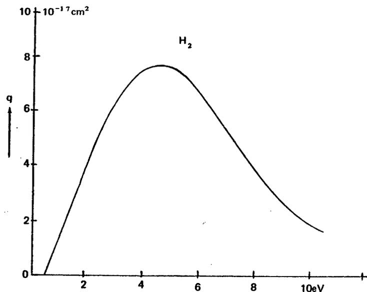
Coarse figure of the excitation cross section for  $\text{H}_2$
