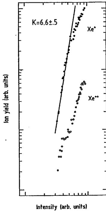
Photoionization of Xe with 100 fs laser pulses
