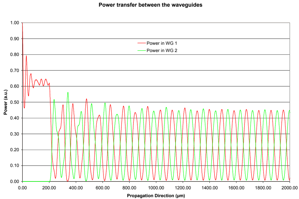
Figure 6.11 Mode power for each waveguide, Waveguide width 1.5\mu\text{m} . Based on Brunner et al. 71
