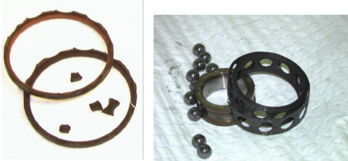
Figure 10. Failure Modes of the Phenolic Cages: (a) Cotton-Phenolic Fails by Thermal Degradation of Matrix and Fibers, and (b) Carbon-Phenolic Fails by Thermal Degradation of the Matrix and Tearing of Carbon Fibers at 30,000 rpm
