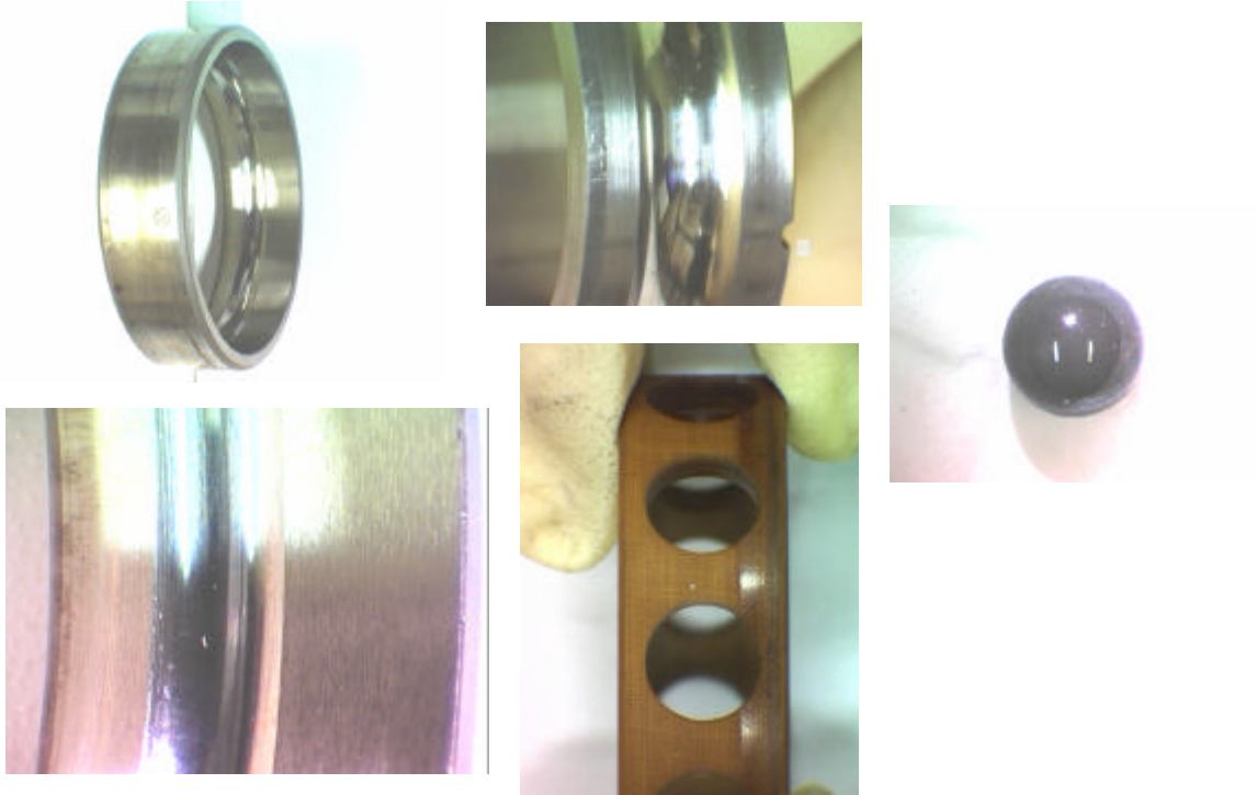
Figure 13. Condition of a Bearing with a Cotton-phenolic Cage after Testing at Shaft Speed of 20,000 rpm
