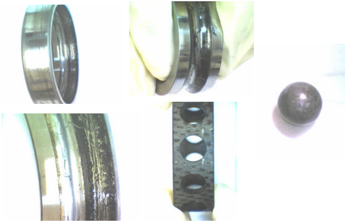
Figure 11. Condition of a Bearing with a Carbon-Phenolic Cage after Testing at Shaft Speed of 20,000 rpm
