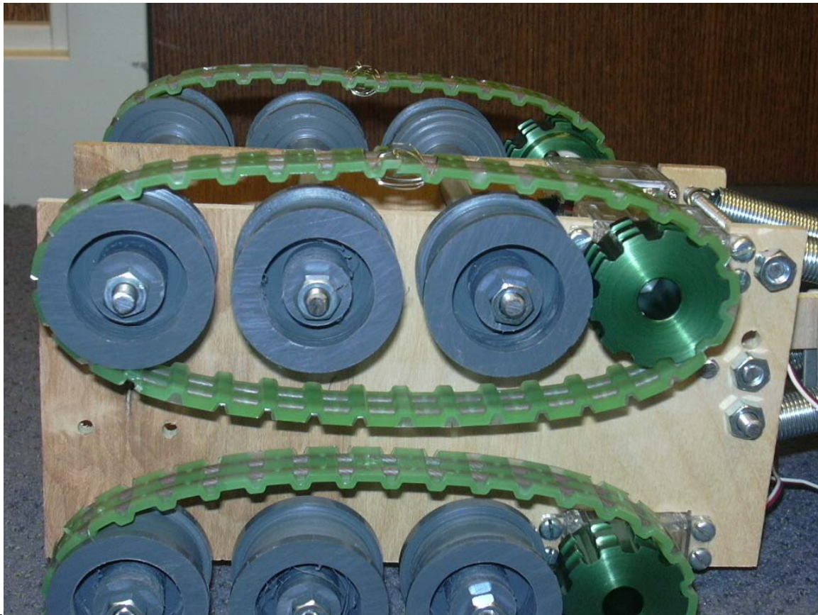
Figure 12: Tread System using W.M.Berg "no-walk" timing belts
