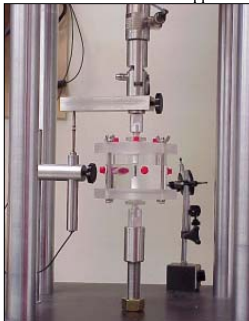
Figure 16: Slow strain rate test rig with specimen immersed in NaCl solution.
