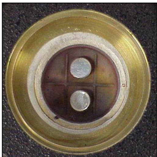
Figure 35: Sample and reference pan used in Differential Scanning Calorimetry (DSC)
