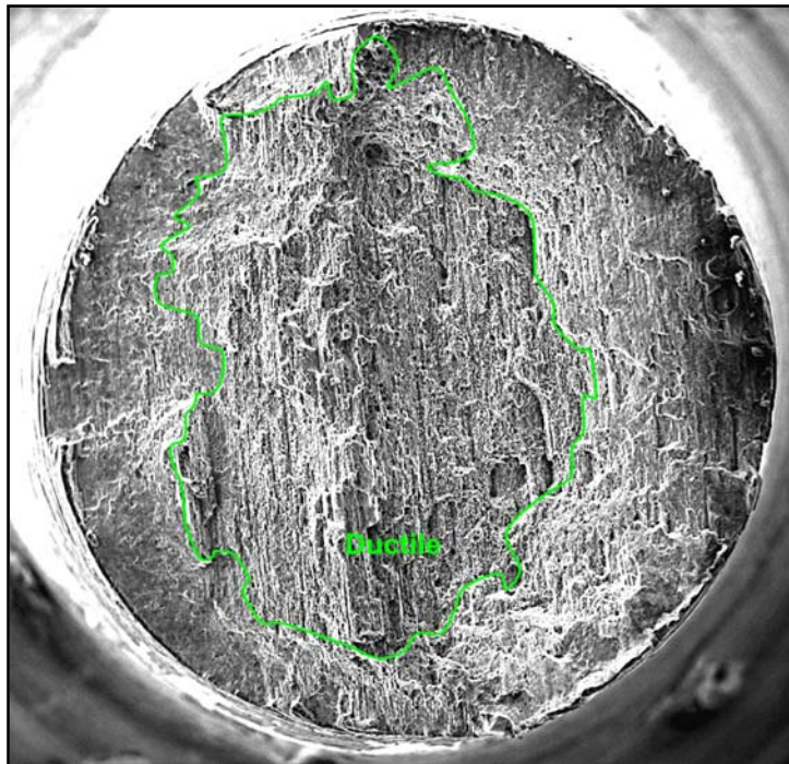
Figure 27: Specimens from 2-inch extrusion stressed perpendicular to the P face in laboratory air (TMRA, above) and 1.0 M NaCl (TMRB, below) [77x].
