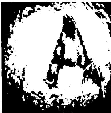
Figure 9 Instantaneous 2-D Image On CCD Array When Depth Is Tuned To The Object (Letter "A") Depth. Image Is Clearly Visible.
