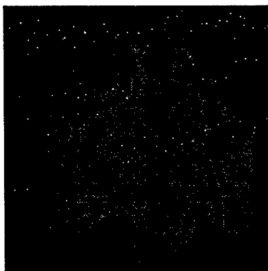
Figure 10 Instantaneous 2-D Image When Depth Is Tuned Off Of Object (Letter "A") Depth. No Image Is Visible On CCD Array.
