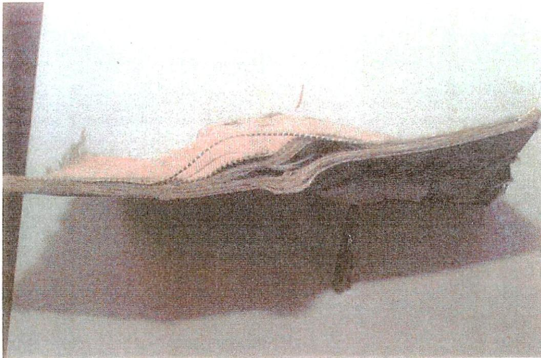
**Figure 2. Cross Section of Delaminated Fiber-Reinforced Plastic**
