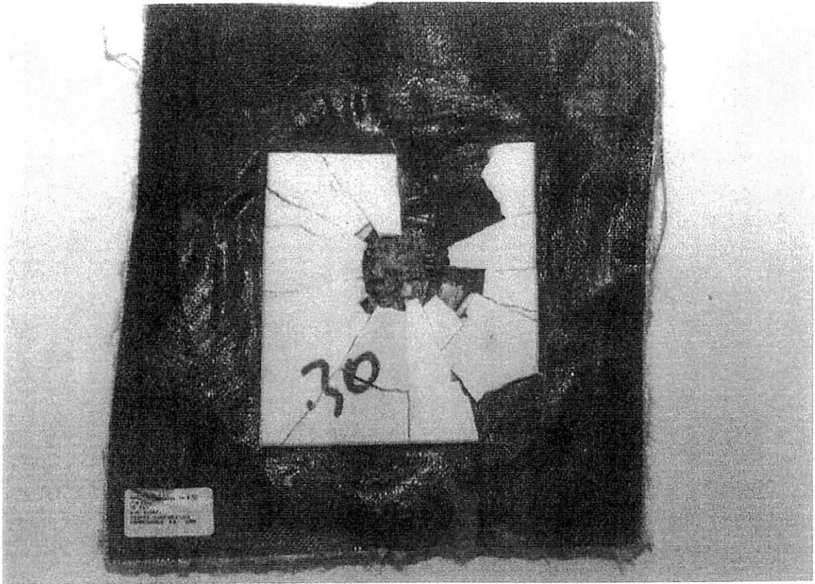
**Figure 1. Ceramic Frontal Component Break-up After Ballistic Impact**
