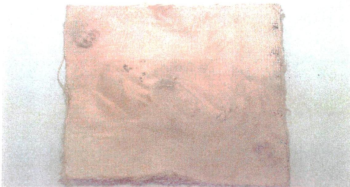
**Figure 3. Rear Surface of Fiber-Reinforced Plastic Surface After Ballistic Impact**
