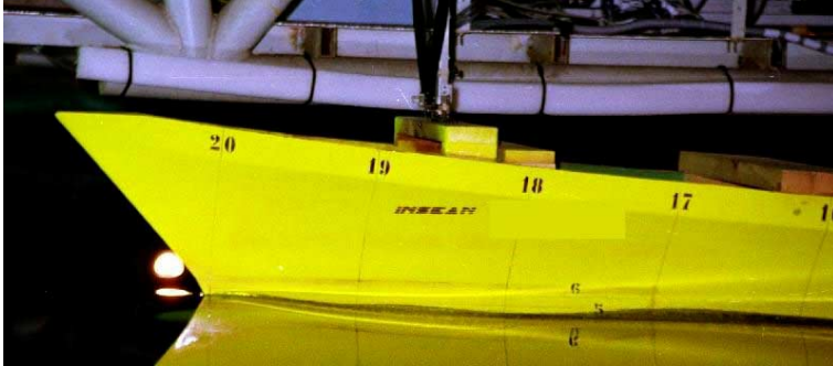
Fig. 10 Experimental verification on the optimal hull shape in the same conditions and viewpoint of fig. 1
