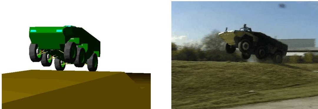
Figure 14: Ramp 1.5m at 40 kph; virtual and physical prototype
