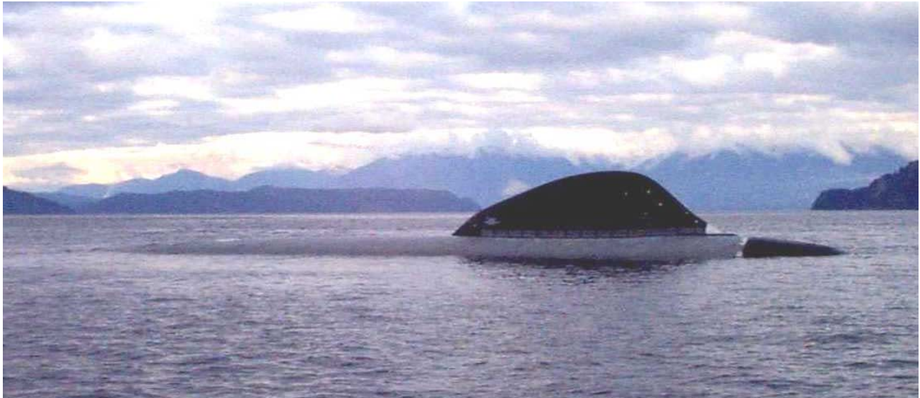
Fig. 14 Advanced Sail installed on the Large Scale Vehicle, from Dozier et al [1].
