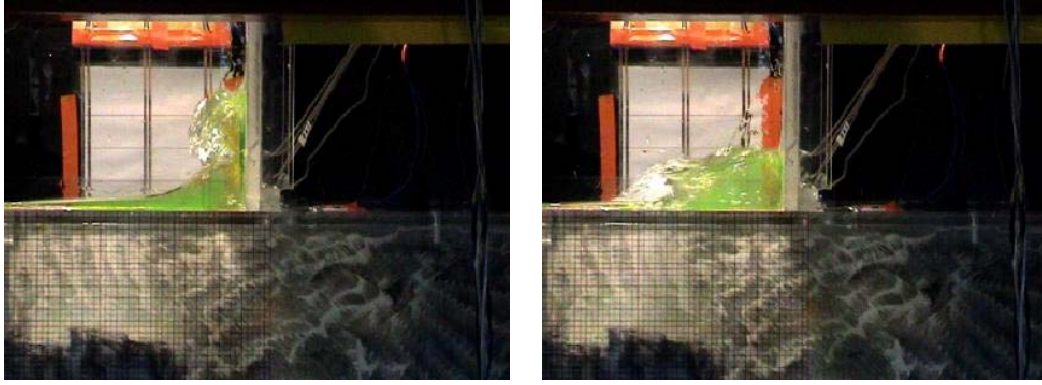
Figure 6. Late evolution of the impact against the vertical superstructure: after the maximum run-up the water plunges backwards onto the deck.
