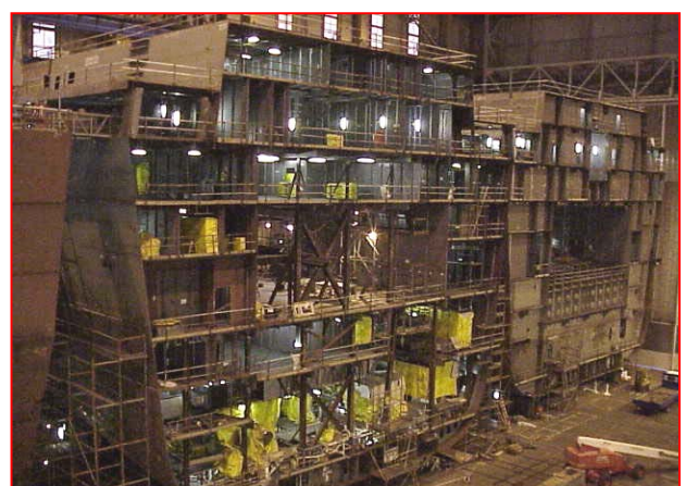
Full block build with advanced stages of outfit
