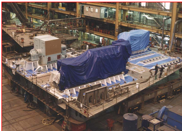
Block Build – All major equipment fitted
