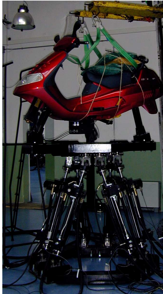
Figure 1 The MORIS motion simulator realized by PERCRO
