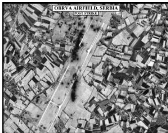
Figure 2. Obrva Airfield, Yugoslavia. Notice the large amount of damage covering both the taxiway and runway and the previous “precision” craters that are filled in.
