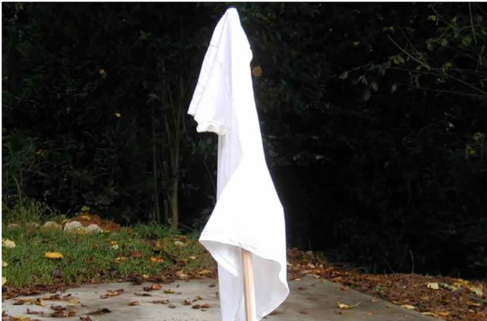
**Figure 31. Tee-shirt draped over the front of the trihedral reflector.**
