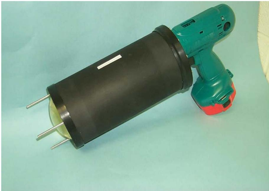
Figure 8. Portable version of the GTRI Radar Flashlight™ sensor.[5]
