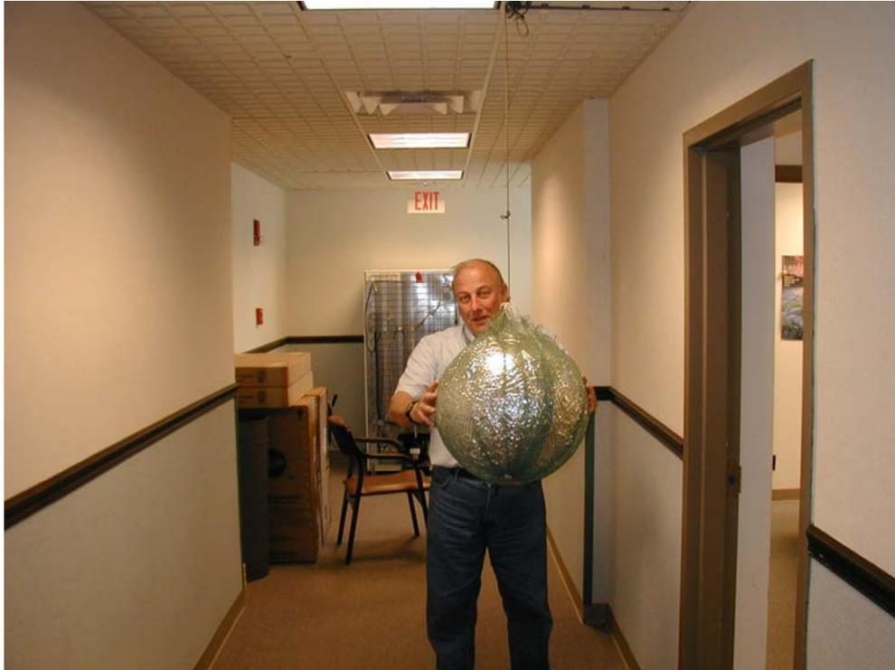
**Figure 15. 18-inch sphere suspended in hallway at Stiefvater Consultants facility for interior concrete wall measurements.**
