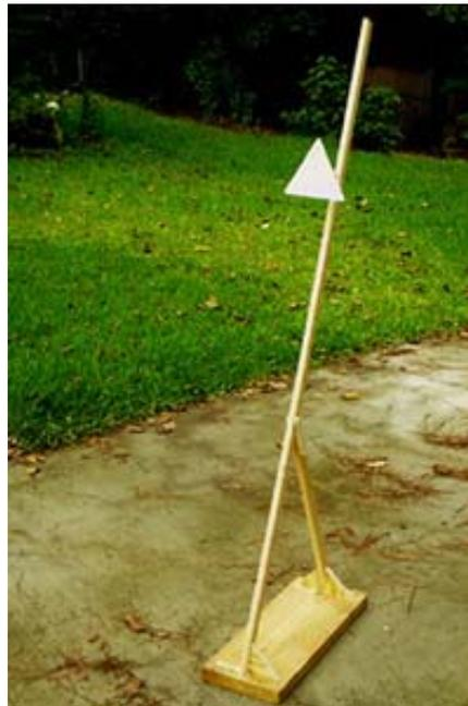
**Figure 25. Reflector/Target test stand.**
