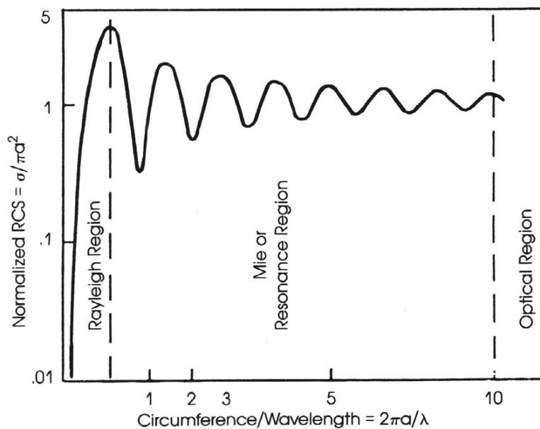
**Figure 13. RCS of a sphere as a function of electrical circumference.[11]**
