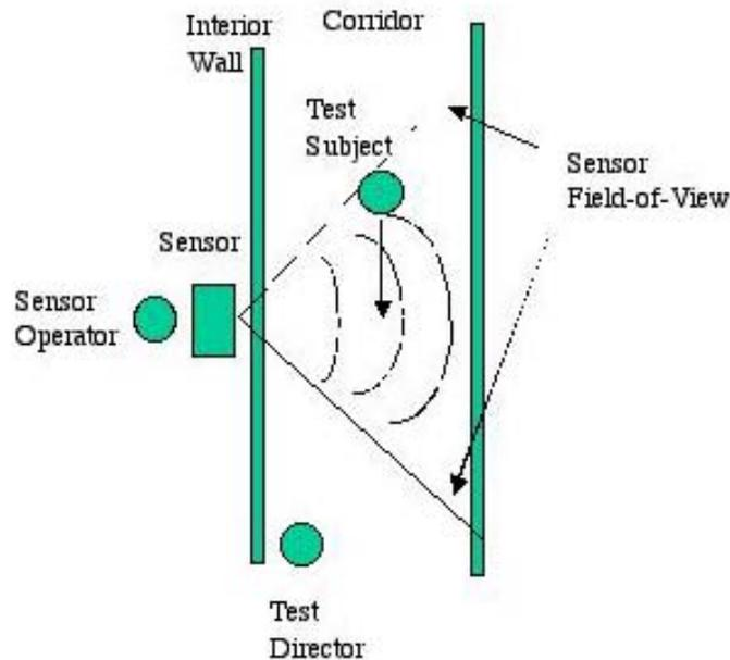
**Figure 16. Representation of “birds eye view” of test scenario for probability of detection and probability of false alarm tests.**
