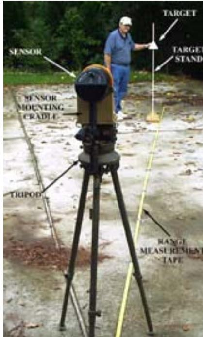
Figure 22. Down-range view of the acoustic measurement range.
