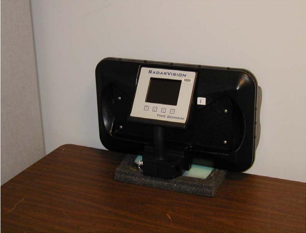
Figure 3. View of Radar Vision 2000 Sensor.
