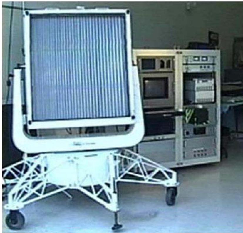
**Figure 1. Trex Enterprises first generation Passive MMW Camera with Bragg cell. [1]**
