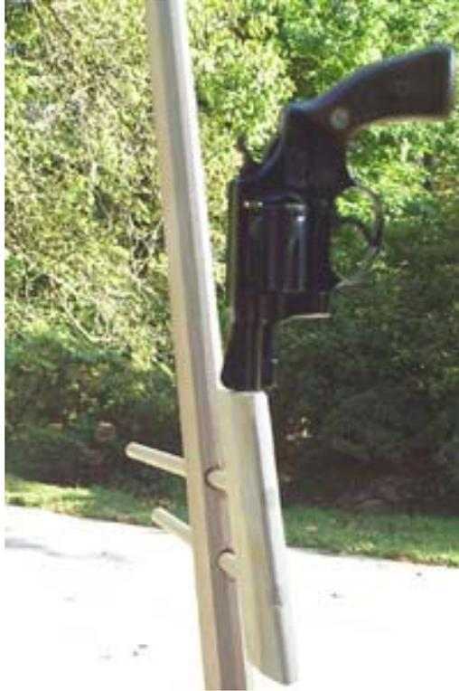
Figure 26. Pistol mounted on test stand fixture.
