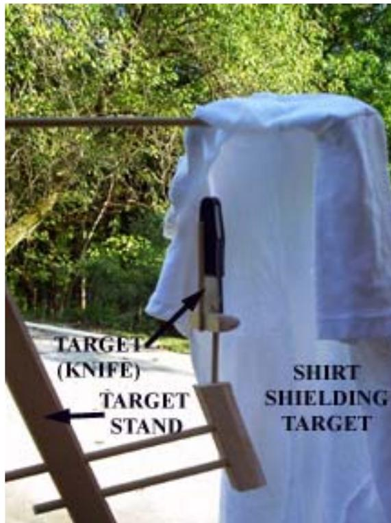
Figure 27. Target on test stand with shirt between sensor and target.
