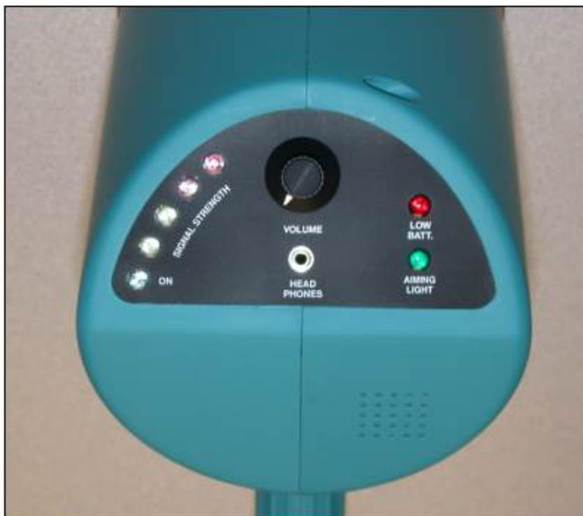
Figure 6. Rear of CWD-2002 showing LEDs.[3]
