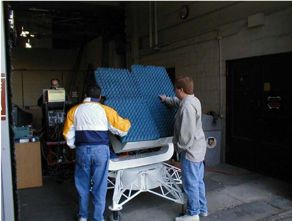
Figure 10. MMW radiometer lens under calibration conditions.
