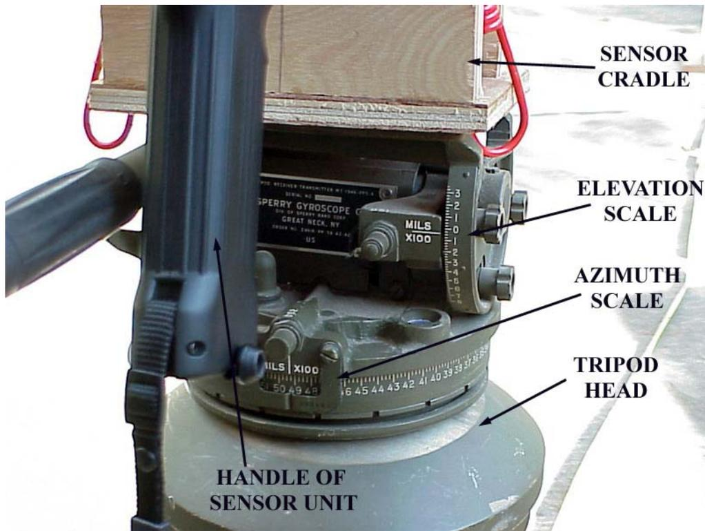
Figure 29. Azimuth and Elevation Scales on tripod head.
