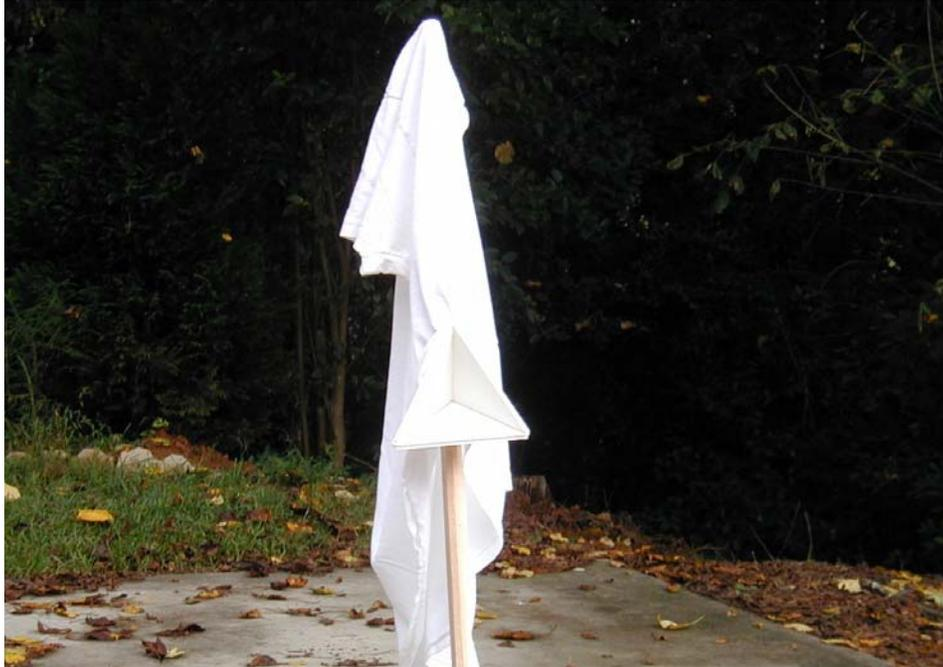
**Figure 30. Tee-shirt draped over top of stand behind the trihedral reflector.**
