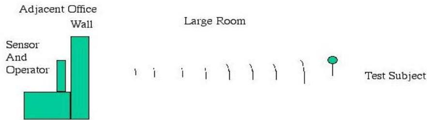
**Figure 9. Scenario for Time Domain probability of detection measurements.**
