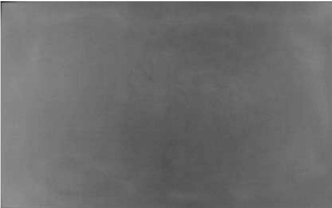
Figure II.23-1. Photograph of black full screen at L_{min} showing luminance nonuniformities and mura on the Samsung 240T LCD monitor.
