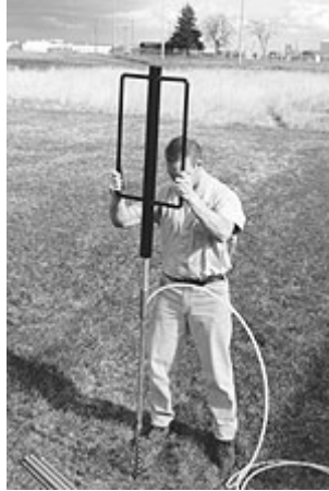
Figure 3-2 Driving Piezometers with a Slide Hammer
