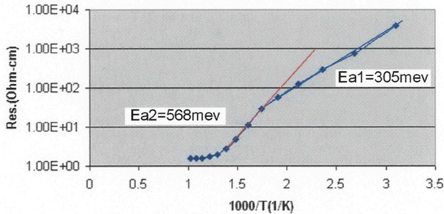
Figure 16. Resistivity versus  $T^{-1}$  obtained on the tail wafer from boule 4.
