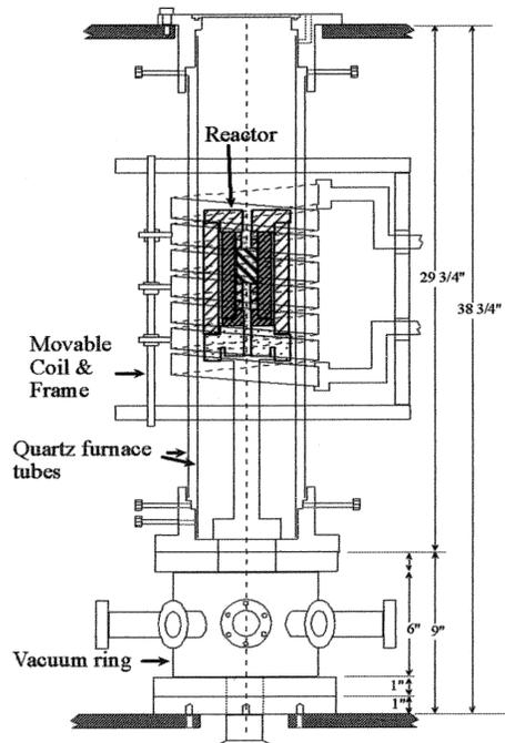
Figure 1. Schematic diagram of the SiC PVT reactor
