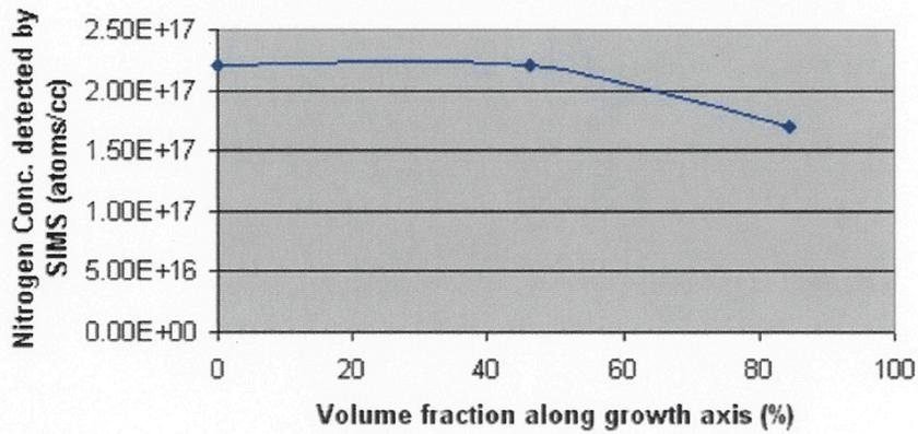
Figure 11 Nitrogen concentration monitored by SIMS in boule 5 as function of fraction of the charge solidified
