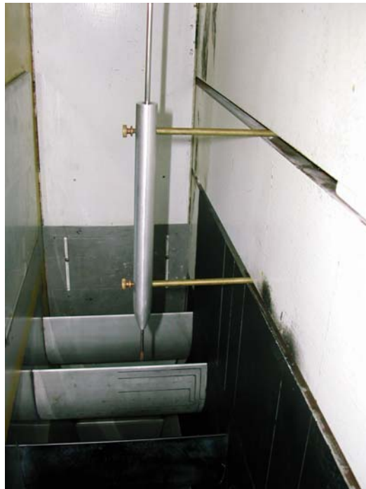
Figure II.5 Probe holder with hot-film probe installed
