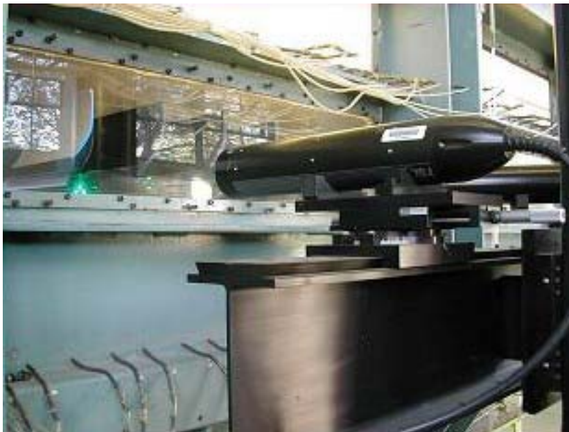
Figure II.8 Inlet-flow angle survey using LDV
