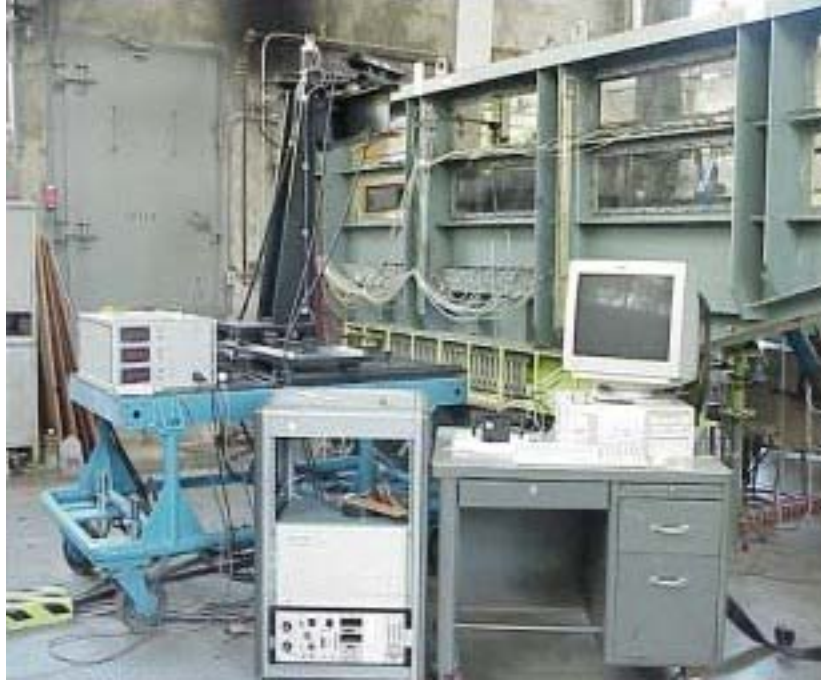
Figure II.7 LDV optics, traverse and data acquisition system
