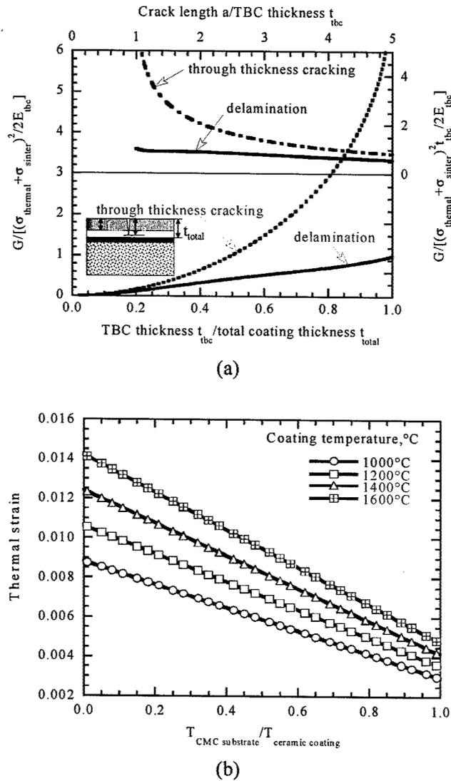
Figure 4.—(a)  $ZrO_2-Y_2O_3$  TBC layer on mullite-BSAS EBC and CMC substrates, the coating surface cracking and delamination energy release rates can increase significantly with a relatively thick, and larger thermal expansion  $ZrO_2-Y_2O_3$  TBC layer on mullite-BSAS EBC on CMC substrates. (b) The significantly larger thermal stresses/strains will be generated with increasing the thermal gradients (the temperature difference between the ceramic coating and the substrates).
