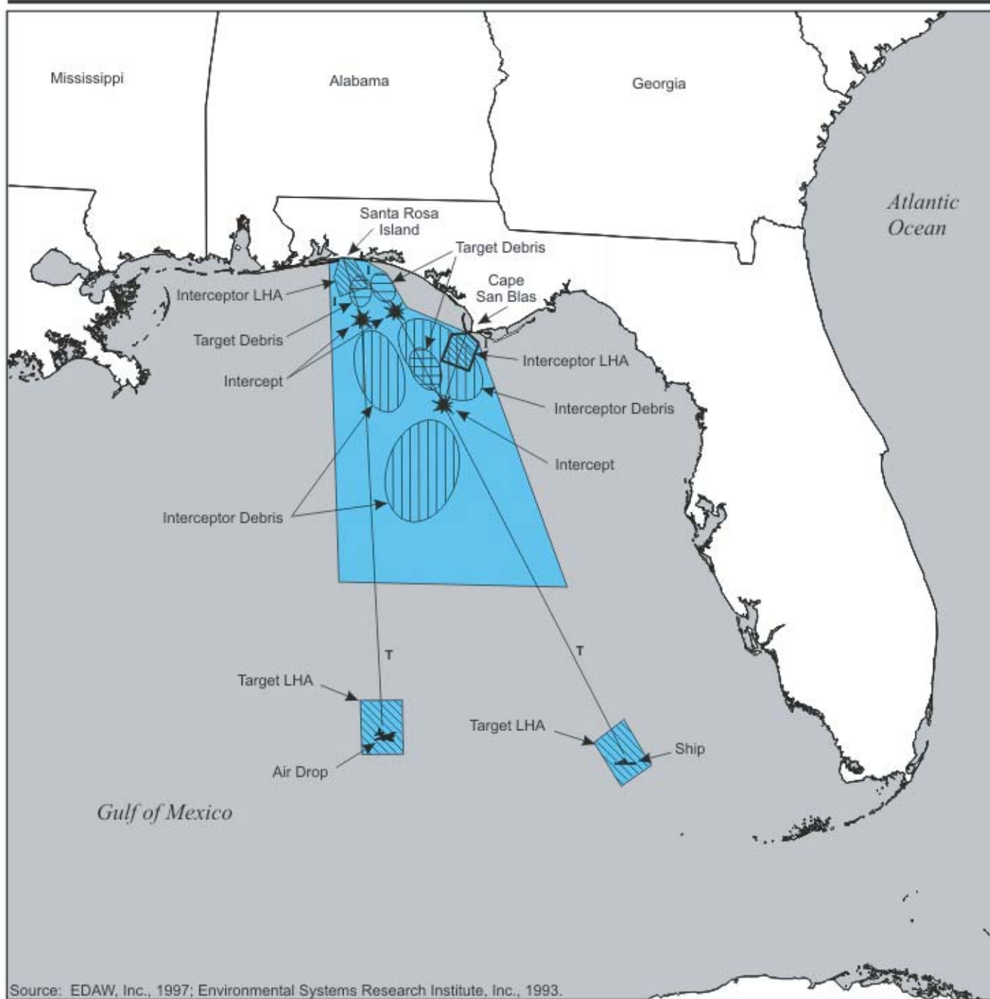
Example 4 - Trajectory of Representative Ship and Air Delivered Targets Intercepted by Multiple Interceptors from Eglin AFB
