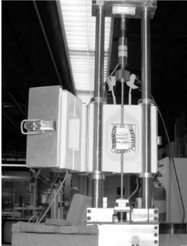
Figure 7. High temperature furnace showing heating coils (center) surrounding pull-rods and grips. A piezoelectric actuator is above the furnace, a capacitance-based load beam below.
